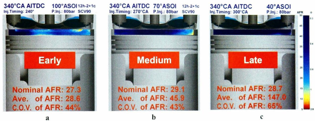
Figure 5.30: Two-dimensional AFR distribution for the 12-hole injector at injection timing of (a). 240°CA, (b).270°CA and (c). 300°CA at 80bar injection pressure and 1,500rpm.
