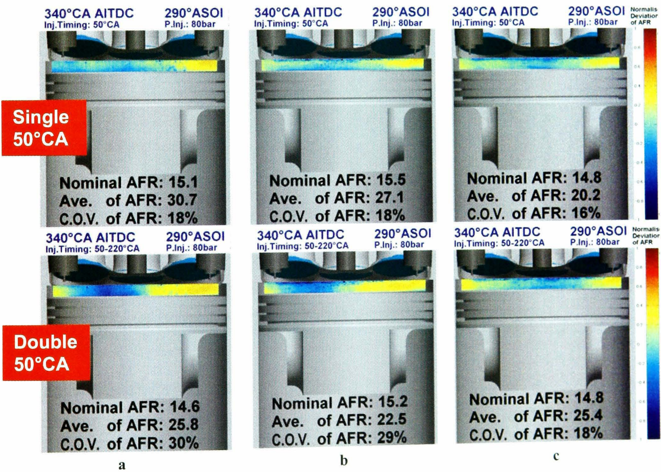
Figure 5.25: Comparison of three different in-cylinder swirl levels for the 12-hole nozzle operating at single- (top row) and double-injection (bottom row) conditions. (a). No swirl (SCV 90°), (b). Medium swirl (SCV 60°) and (c). Maximum swirl (SCV 0°) at 50°CA injection timing.
