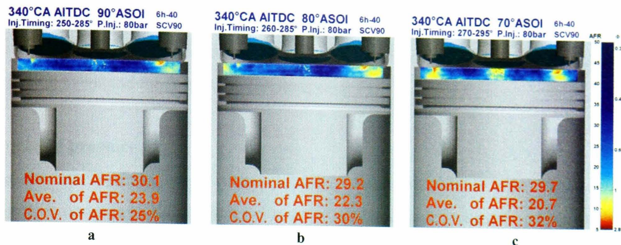
Figure 5.38: Two-dimensional AFR distribution for the 6-hole injector at double-injection strategy. Injection timings of (a). 250-285°CA, (b).260-285°CA and (c). 270-295°CA at 80bar injection pressure and 3,000rpm.
