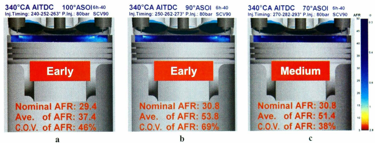
Figure 5.35: Two-dimensional AFR distribution for the 6-hole injector at triple-injection strategy. Injection timings of (a). 240-252-263°CA, (b).250-262-273°CA and (c). 270-282-293°CA at 80bar injection pressure and 1,500rpm.
