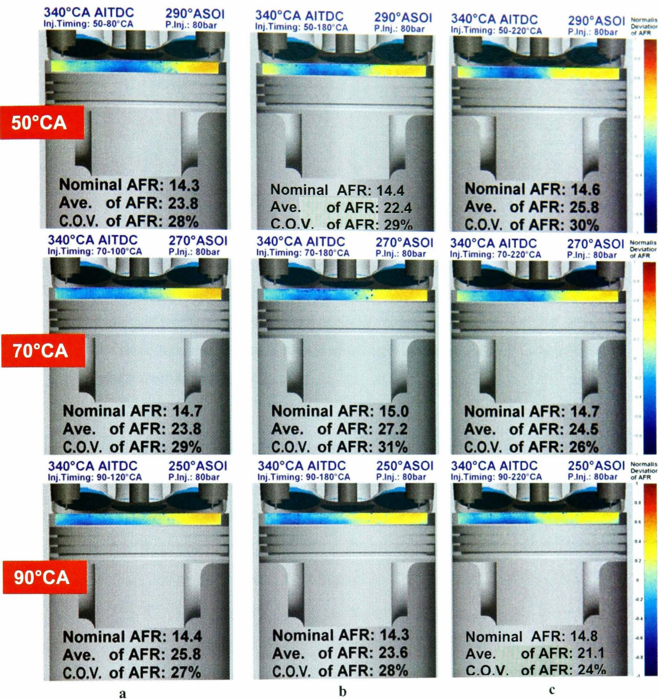
Figure 5.18: Two-dimensional deviation of air/fuel ratio (AFR) distribution at 340°C AITDC (20° before compression TDC) of the 12-hole injector at double-injection strategy. The timing of the first injection in the sequence is set at 50°C CA (top row), at 70°C CA (middle row) and at 90°C CA (bottom row). The second injection timing is placed at (a). 30°CA after the start of the first injection event, (b). 180°CA, or bottom dead centre and (c). 220°CA, timing at which inlet valves have closed.
