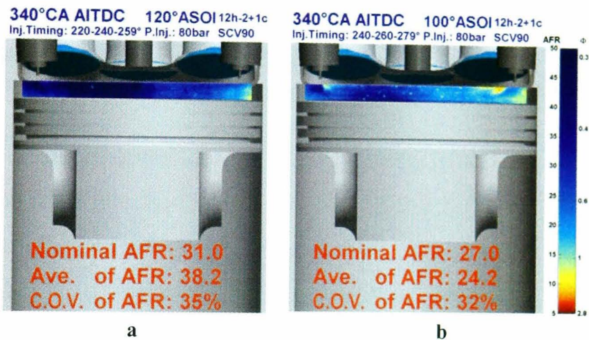
Figure 5.37: Two-dimensional AFR distribution for the 12-hole injector at triple-injection strategy. Injection timings of (a). 220-240-260°CA and (b).240-260-279°CA at 80bar injection pressure and 3,000rpm.
