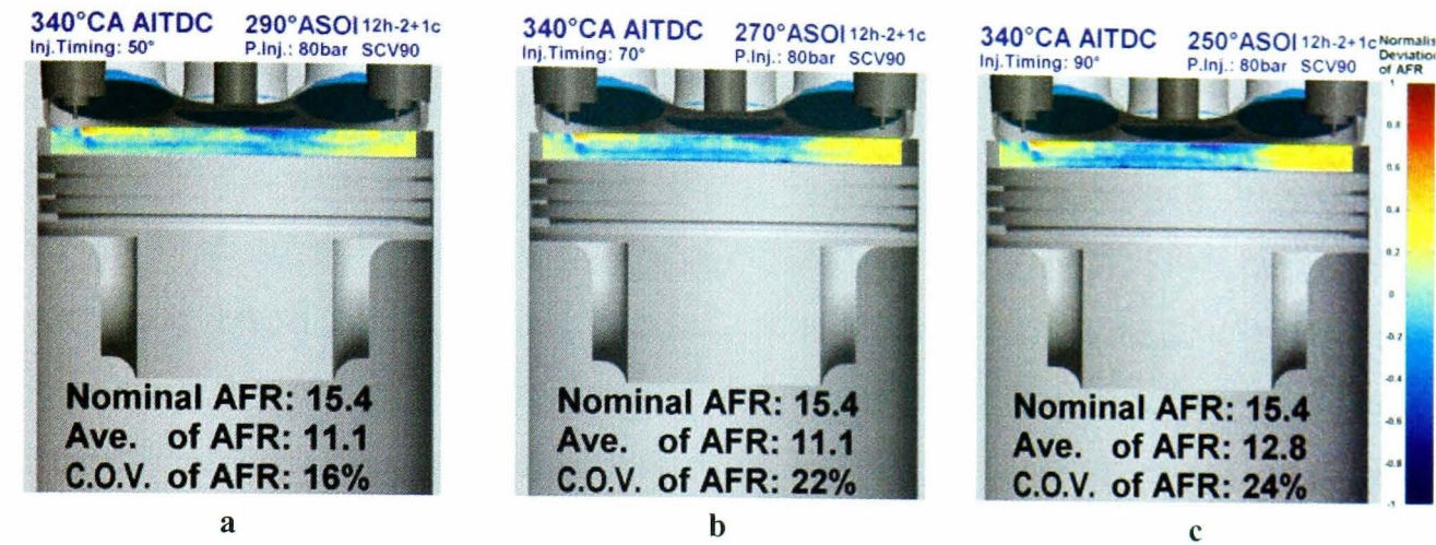
Figure 5.16: Two-dimensional deviation of air/fuel ratio (AFR) distribution at 340°CA (20° before compression TDC) of the 12-hole injector at injection timings of (a). 50°, (b). 70° and (c). 90°CA.
