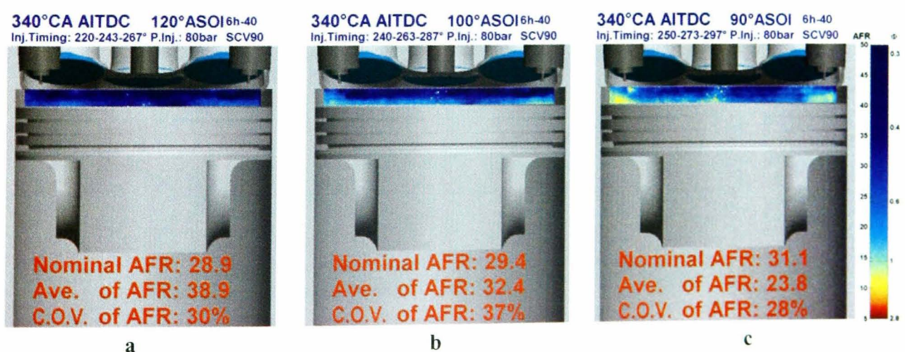
Figure 5.39: Two-dimensional AFR distribution for the 6-hole injector at triple-injection strategy. Injection timings of (a). 220-243-257°CA, (b).240-253-287°CA and (c). 250-273-297°CA at 80bar injection pressure and 3,000rpm.
