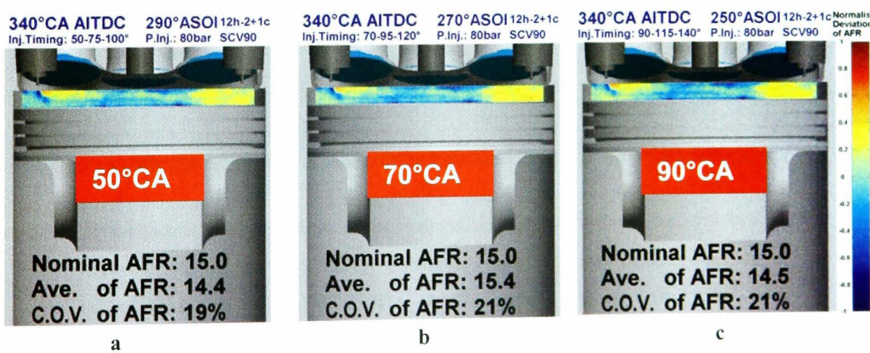
Figure 5.23: Two-dimensional deviation of air/fuel ratio (AFR) distribution at 340°CA (20° before compression TDC) of the 12-hole injector at triple-injection strategy. Injection timings of (a). 50-90-120°CA, (b). 70-110-140°CA and (c). 90-130-160°CA.
