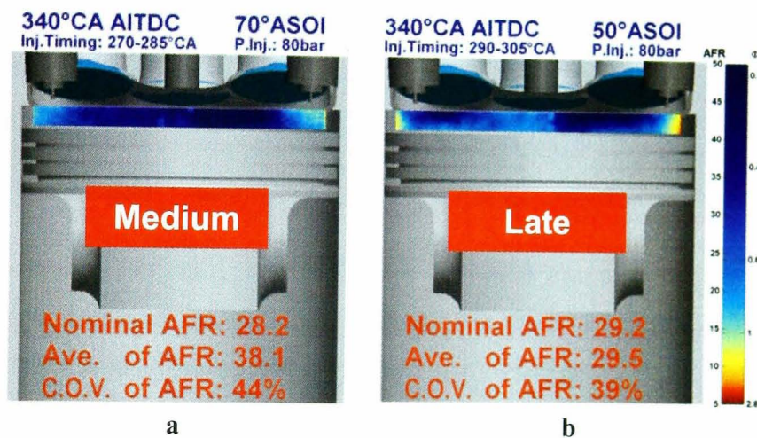
Figure 5.34: Two-dimensional AFR distribution for the 6-hole injector at double-injection strategy. Injection timings of (a). 270-285°CA and (b). 290-306°CA at 80bar injection pressure and 1,500rpm.
