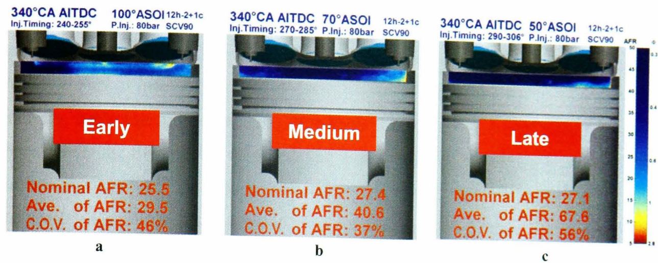
Figure 5.33: Two-dimensional AFR distribution for the 12-hole injector at double-injection strategy. Injection timings of (a). 240-255°CA, (b).270-285°CA and (c). 290-306°CA at 80bar injection pressure and 1,500rpm.
