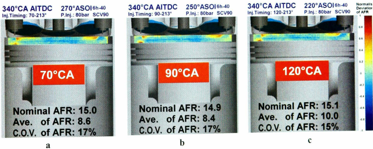
Figure 5.24: Two-dimensional deviation of air/fuel ratio (AFR) distribution at 340°C AITDC (20° before compression TDC) of the 6-hole injector at double-injection strategy. Injection timings of (a). 70-213°CA, (b). 90-213°CA and (c). 120-213°CA.
