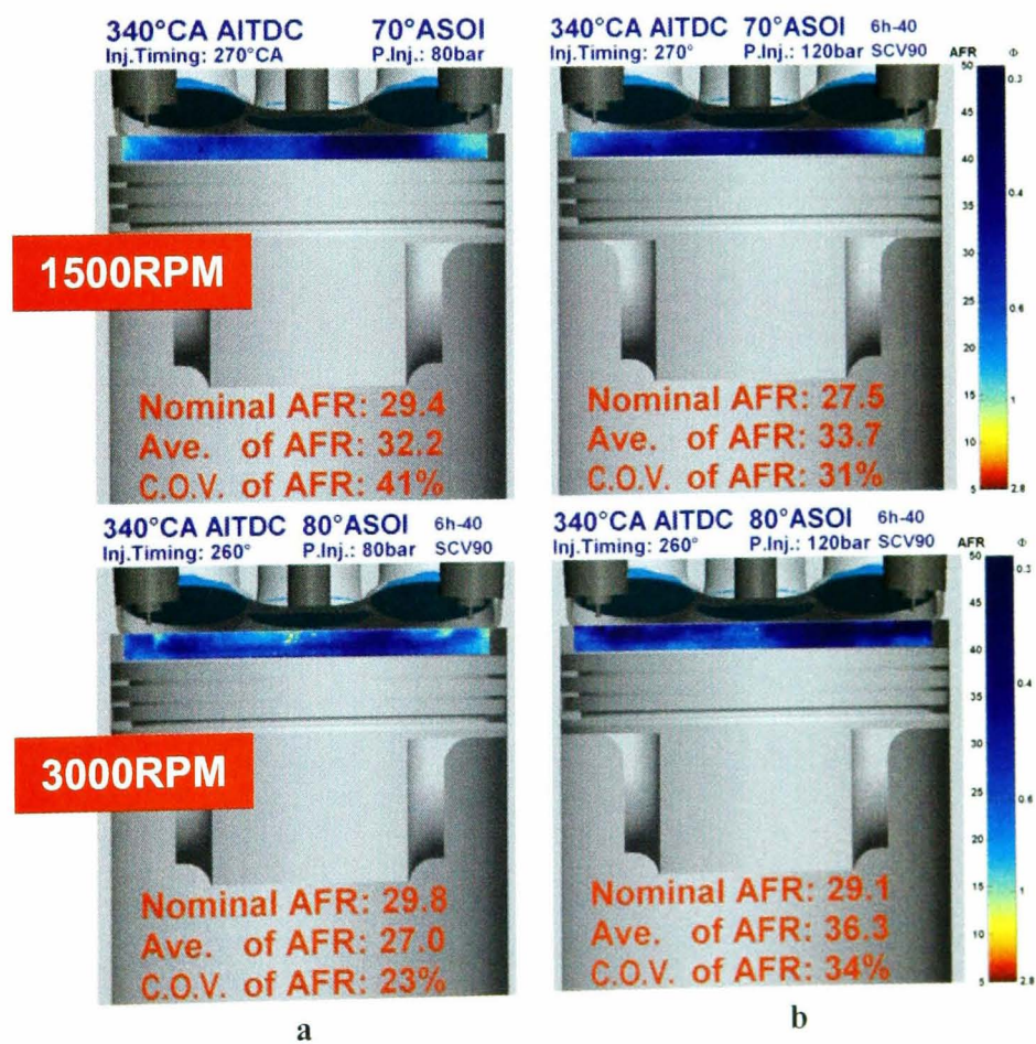
Figure 5.40: Two-dimensional AFR distribution for the 6-hole injector at low (1,500rpm – top row) and high (3,000rpm – bottom row) engine speed. Injection pressure of (a). 80bar and (b). 120bar at two different injection timings.
