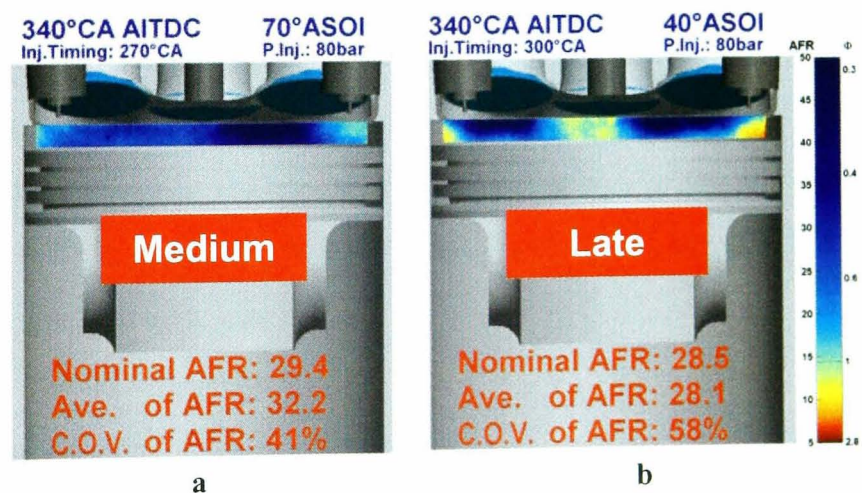
Figure 5.31: Two-dimensional AFR distribution for the 6-hole injector at injection timing of (a). 270°CA and (b). 300°CA at 80bar injection pressure and 1,500rpm.
