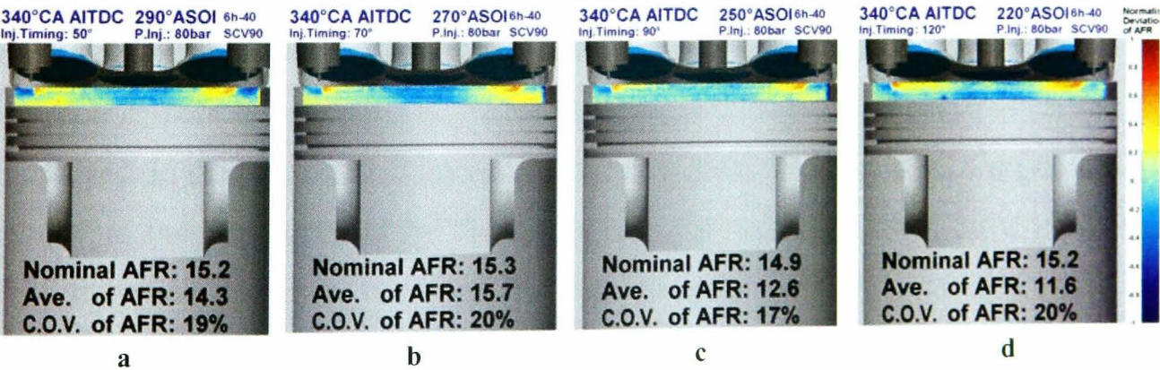
Figure 5.17: Two-dimensional deviation of air/fuel ratio (AFR) distribution at 340°CA (20° before compression TDC) of the 6-hole injector at injection timings of (a). 70°, (b). 90° and (c). 120°CA.
