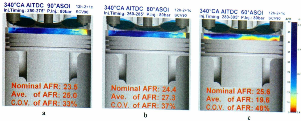
Figure 5.36: Two-dimensional AFR distribution for the 12-hole injector at double-injection strategy. Injection timings of (a). 250-275°CA, (b).260-285°CA and (c). 280-305°CA at 80bar injection pressure and 3,000rpm.
