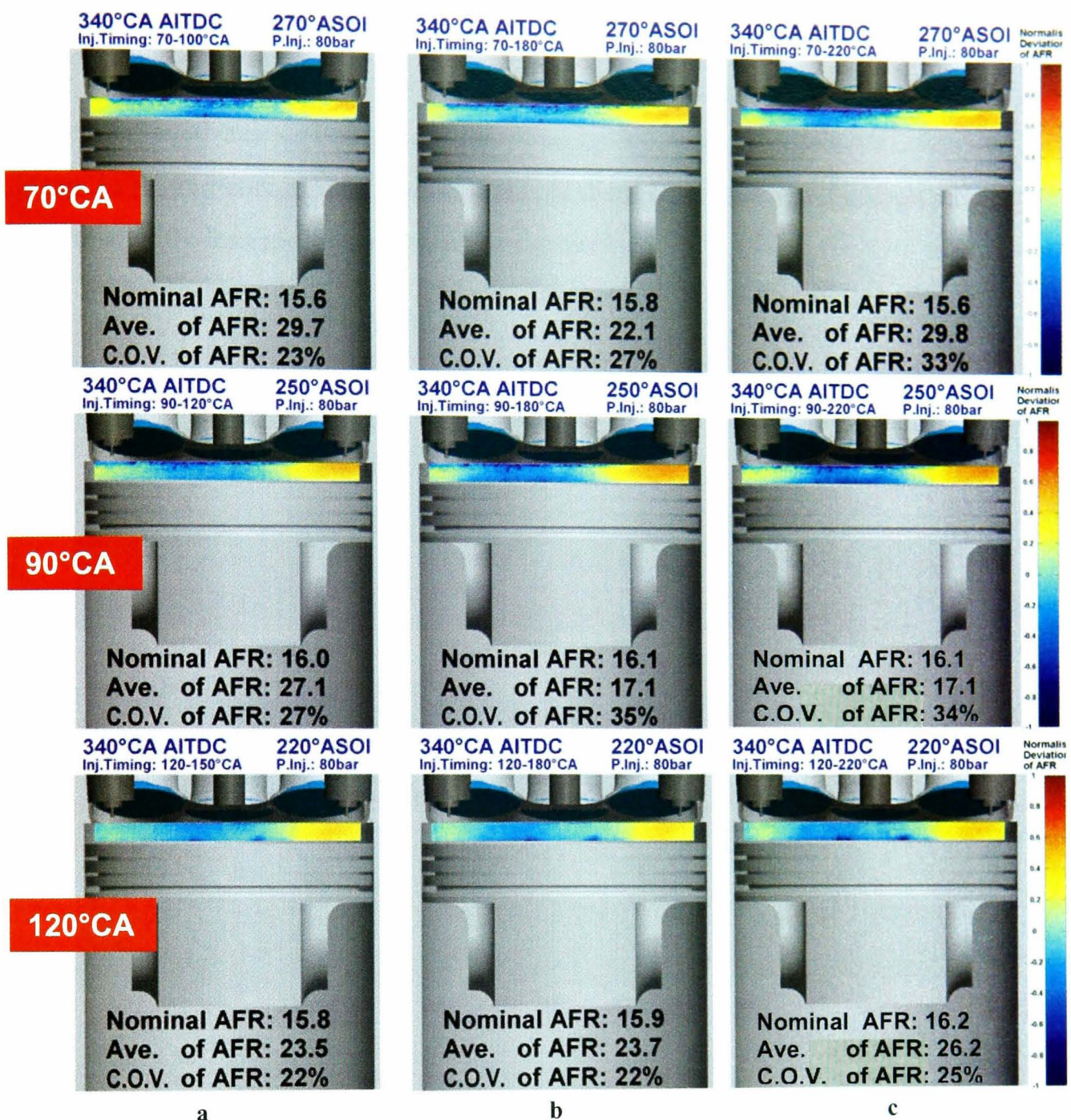
Figure 5.20: Two-dimensional deviation of air/fuel ratio (AFR) distribution at 340°C AITDC (20° before compression TDC) of the 6-hole injector at double-injection strategy. The timing of the first injection in the sequence is set at 70°C CA (top row), at 90°C CA (middle row) and at 120°C CA (bottom row). The second injection timing is placed at (a). 30° CA after the start of the first injection event, (b). 180° CA, or bottom dead centre and (c). 220° CA, timing at which inlet valves have closed.
