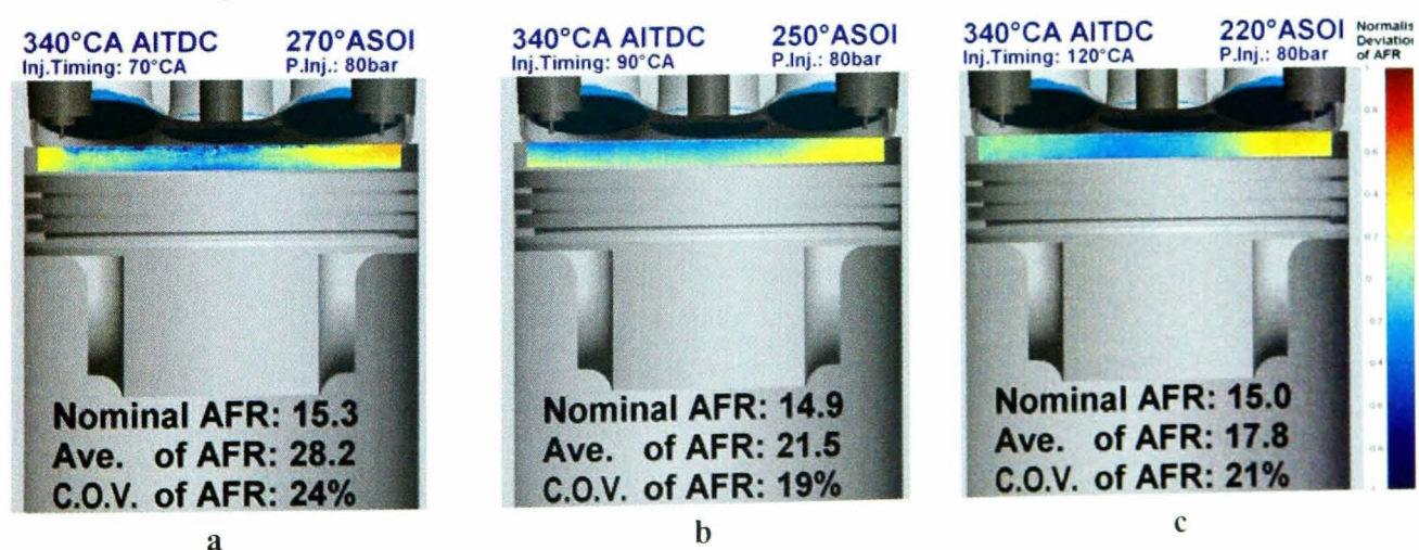
Figure 5.14: Two-dimensional deviation of air/fuel ratio (AFR) distribution at 340^\circ\text{CA} ( 20^\circ before compression TDC) of the 6-hole injector at injection timings of (a). 70^\circ , (b). 90^\circ and (c). 120^\circ\text{CA} .
