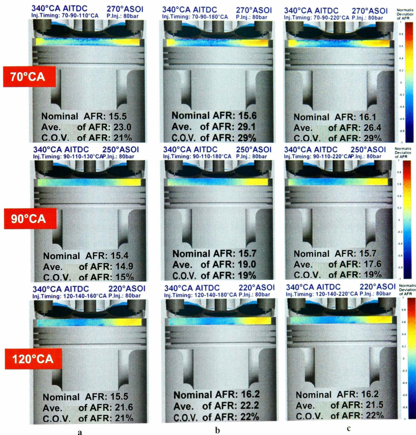
Figure 5.21: Two-dimensional deviation of air/fuel ratio (AFR) distribution at 340^{\circ}\text{CA} ( 20^{\circ} before compression TDC) of the 6-hole injector at triple-injection strategy. The timing of the first injection in the sequence is set at 70^{\circ}\text{CA} (top row), at 90^{\circ}\text{CA} (middle row) and at 120^{\circ}\text{CA} (bottom row). The second at 20^{\circ}\text{CA} after the start of the first pulse and the third injection timing is placed at (a), 20^{\circ}\text{CA} after the start of the second pulse, (b), 180^{\circ}\text{CA} or bottom dead centre and (c), 220^{\circ}\text{CA} , timing at which inlet valves have closed.
