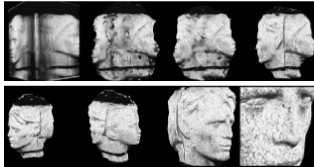
Figure 8. Reconstruction (above) and new view synthesis (below) of a two-headed object using the level set method. Images courtesy of Olivier Faugeras and Renaud Keriven.
