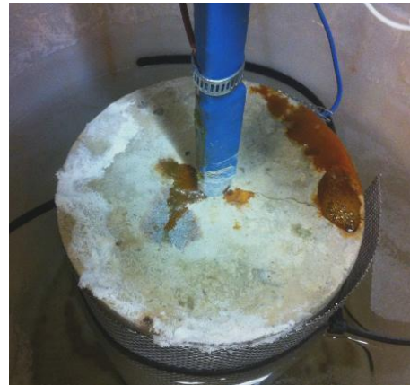
Fig. 8 Photo of corroding cylinder
