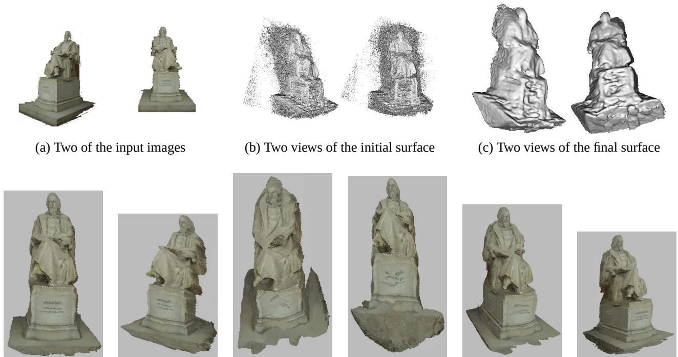
Figure 2. Reconstruction of Lord Tennyson statue. The top row shows two of the input images followed by views of the initial and final surface. The bottom row shows many more views of the final reconstruction with texture mapping of the original image data.
