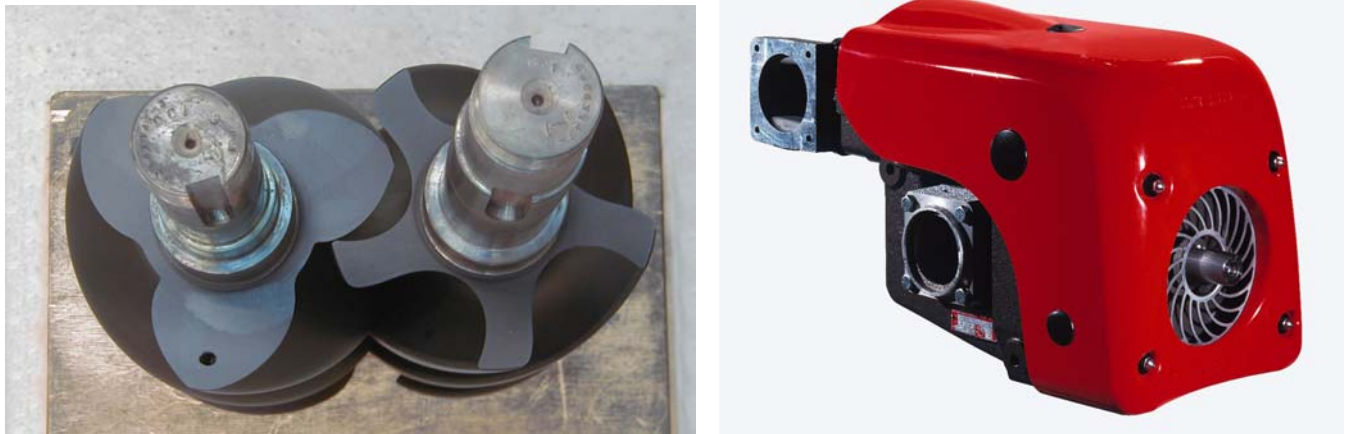
Fig. 3 Rotor profile for delivery of dry air, McCreath et al, 2001
