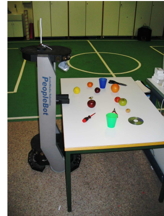
Figure 1. The robot standing in front of a white table. Different objects are laying on the table. The robot has to grasp or point to objects specified in simple command sentences.
