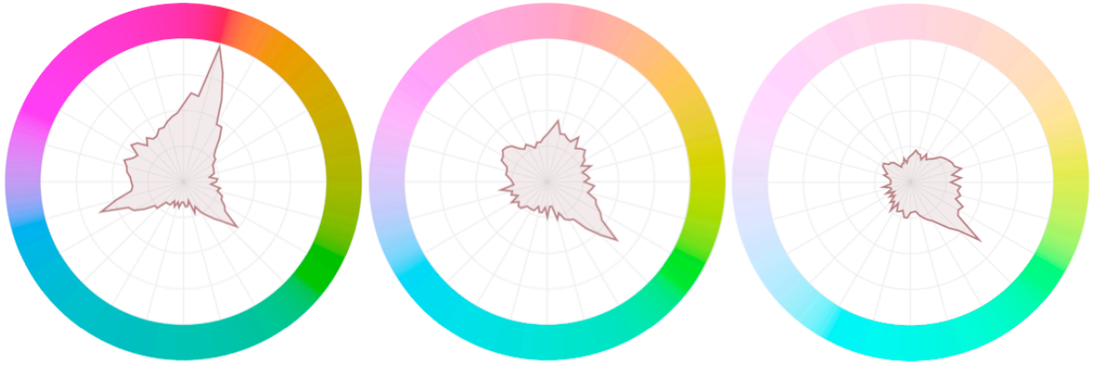
Figure 1: Graphs showing the ease of hue discrimination at lightnesses of 30%, 50% and 70% (left to right). Distance from the centre of each graph is proportional to degree of perceptual discrimination of the given hue.
