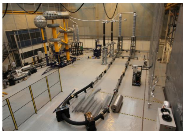
Fig. 20. HVDC cable ageing facility at Alstom Grid, Stafford, UK
