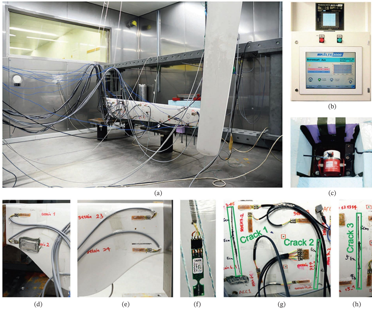
FIGURE 1 | Summary of the experimental campaign elements: (a) blade inside the climate chamber; (b) climate controller; (c) electromechanical shaker; (d, e) strain gauges on the low- and high-pressure sides; (f) climate sensor; (g, h) introduced cracks [18].
