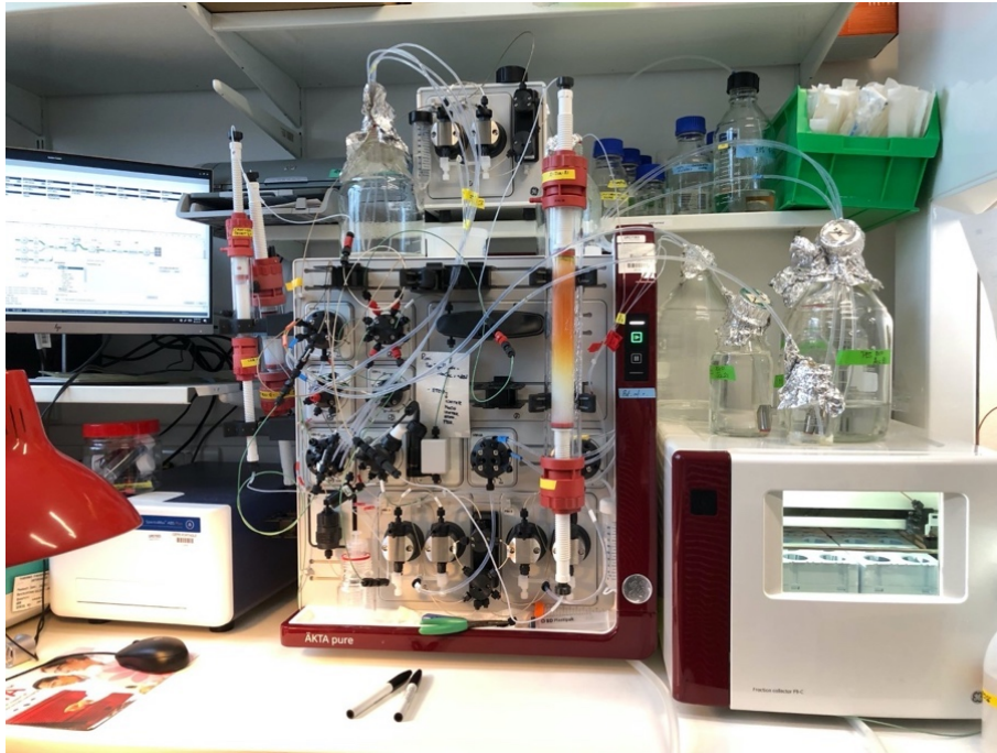
Image 2.3. Sterile purification of cord blood plasma, applied to chromatography system with attached IgG and IgM depletion columns.
