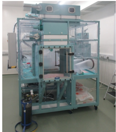
Image 2.4. Flexible film isolator in a category three laboratory (left).
