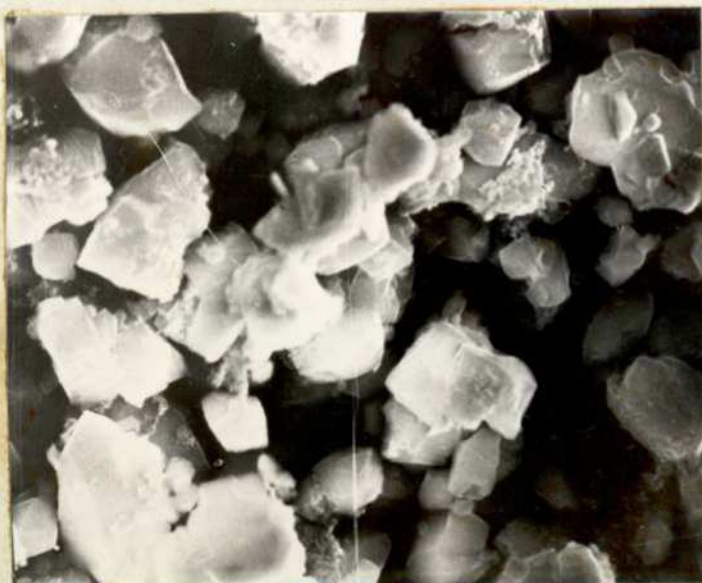
Figure 6.13 Discharged \text{Cd}(\text{OH})_2 Electrode after 3 Standard Cycles.
