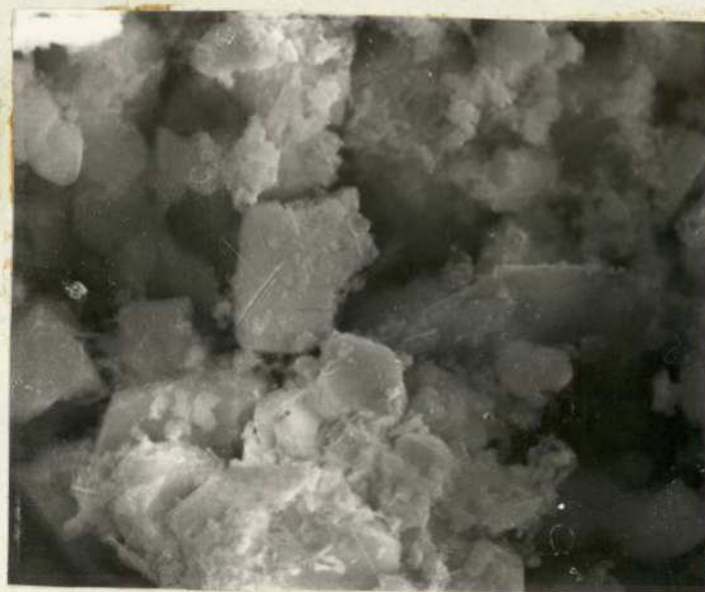
Figure 6.2 New Negative after the 8th C/40 discharge Cycle and Room Temperature.
