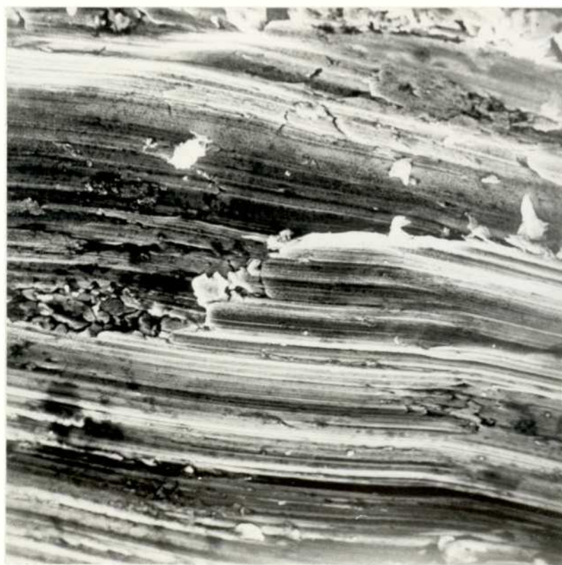
FIGURE 34: SCANNING ELECTRON MICROGRAPH STAINLESS STEEL EN58B—KNURLED ROLLERS
