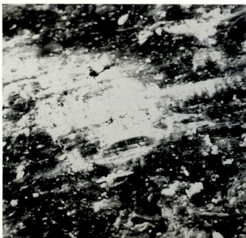
FIGURE 37: SCANNING ELECTRON MICROGRAPH MILD STEEL CR4 — PLAIN ROLLERS
