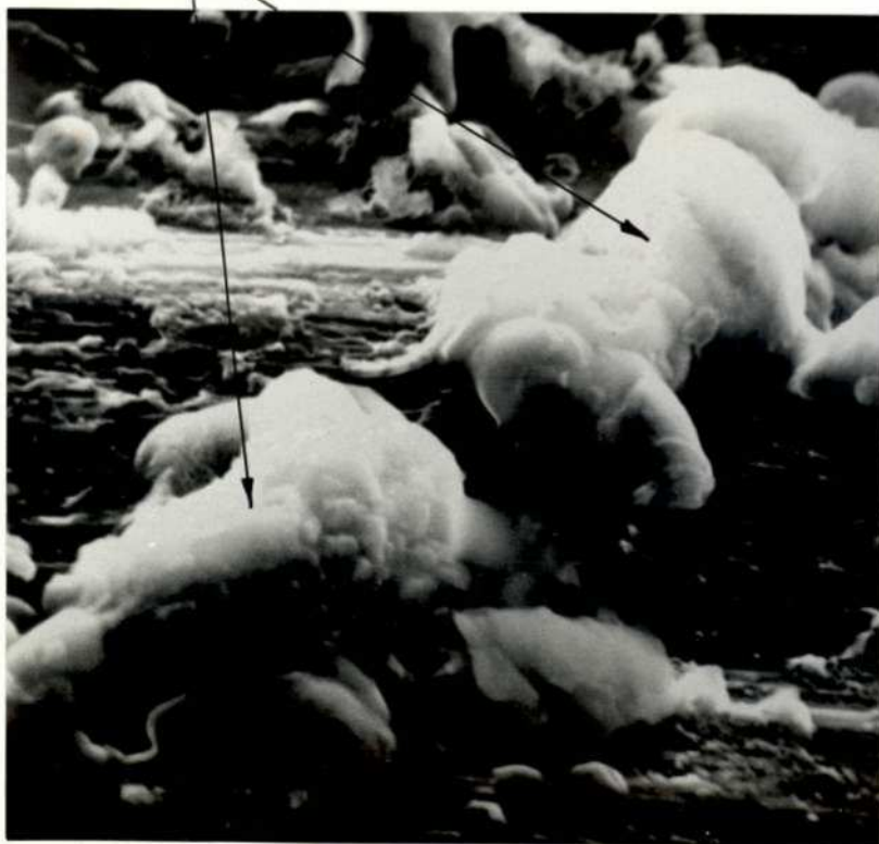
FIGURE 36: SCANNING ELECTRON MICROGRAPH 70/30 BRASS — KNURLED ROLLERS
