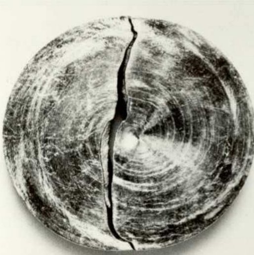
(c) FRACTURED ALUMINIUM ALLOY SPECIMEN R = 0.15 , F_E = 273 \text{ kN} , \theta = 10^\circ
