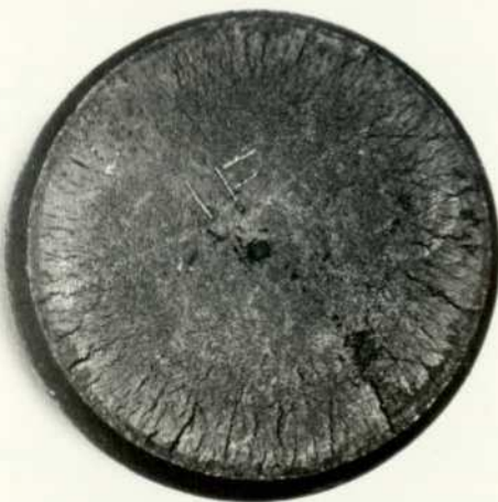
(b) Typical post-sintered iron powder metal specimens D_0 = 30 mm, H_0/D_0 = 0.66 after fractional reduction in height caused by warm upsetting
