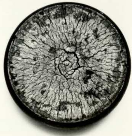
(b) Typical post-sintered iron powder metal specimens D_0 = 30 mm, H_0/D_0 = 0.66 after fractional reduction in height caused by warm upsetting
