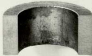
(c) Typical satisfactory post-sintered iron powder metal hollow cylindrical specimens of 30 mm external diameter.
