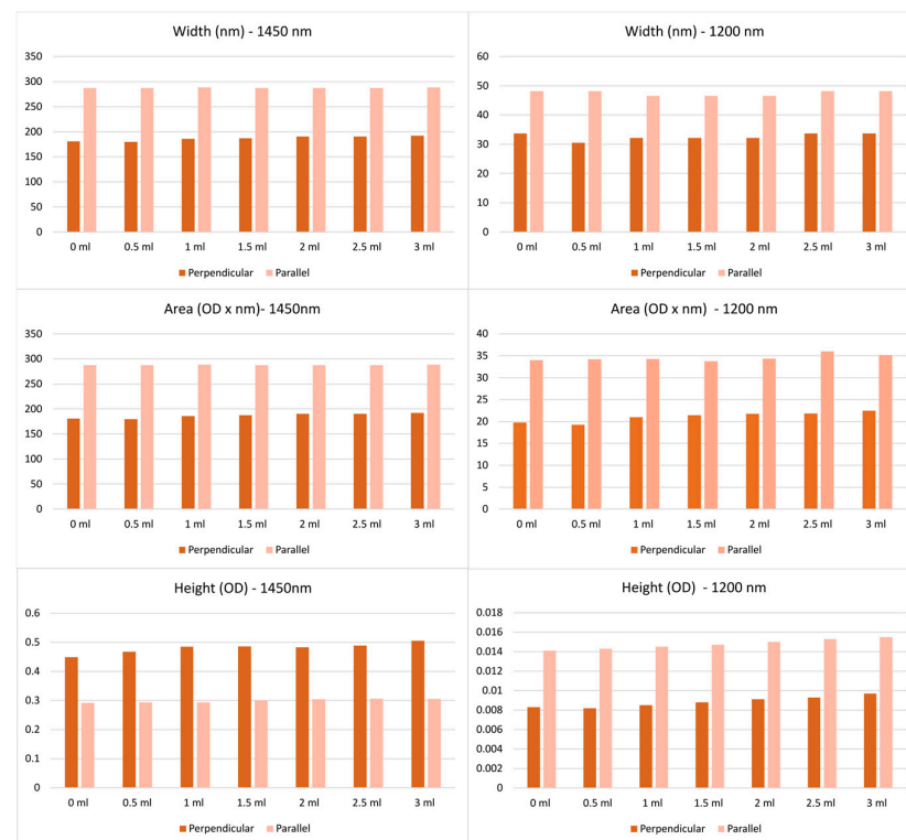
Figure 5. Height, width, and area under the curve for perpendicular and parallel measurements across different fluid volumes (0–3 mL, in 0.5 mL increments) at 1200 nm and 1450 nm. Top row: width measurements (nm); middle row: area (OD × nm); bottom row: height (OD). The left column corresponds to 1450 nm and the right column to 1200 nm. OD = optical density.
