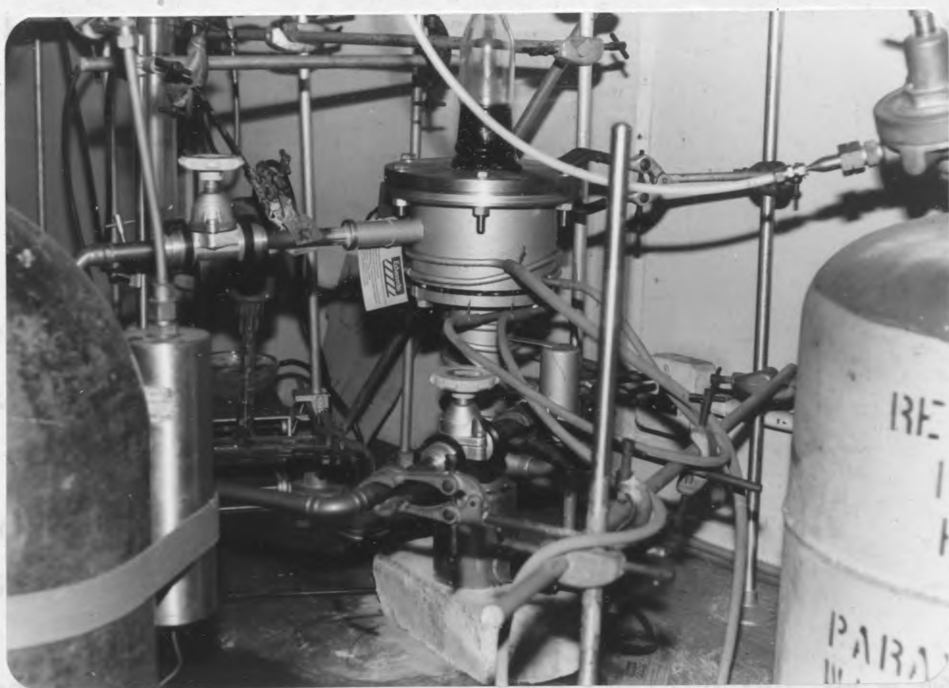
Plate 6 Diffusion pump showing muff-coupled valves
