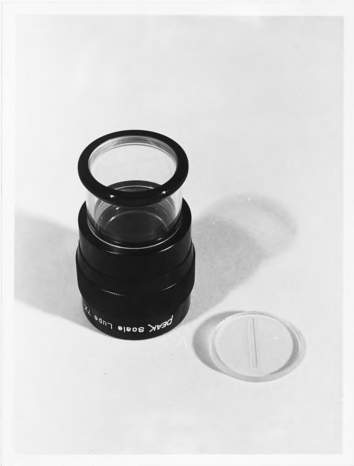
Figure 4.13. Measuring magnifier used for HVID measurements on negatives.
