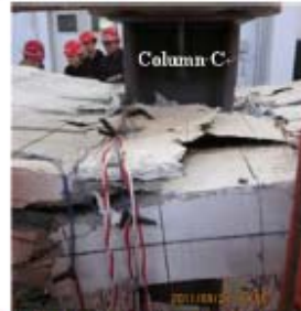
f) Crushing around column C
