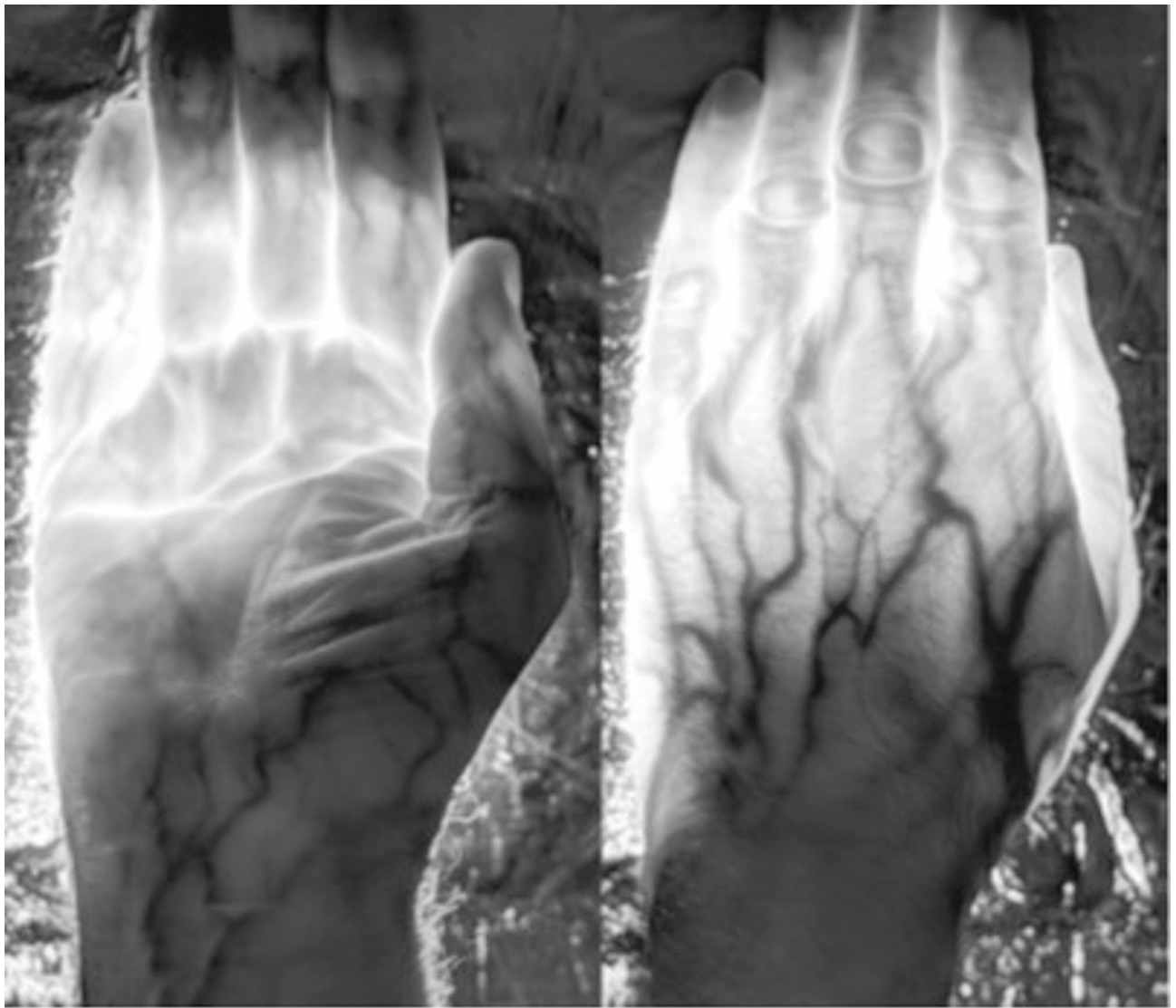
Fig. 4. Light transmission through the hand from an 850 nm LED source. Because the tissues are relatively thin compared with the thorax it was possible to map the spectrum here against known biological absorbers. The images clearly show that deoxygenated blood is a key absorber. Also, bone can not be seen and hence is relatively transparent at these longer wavelengths.
