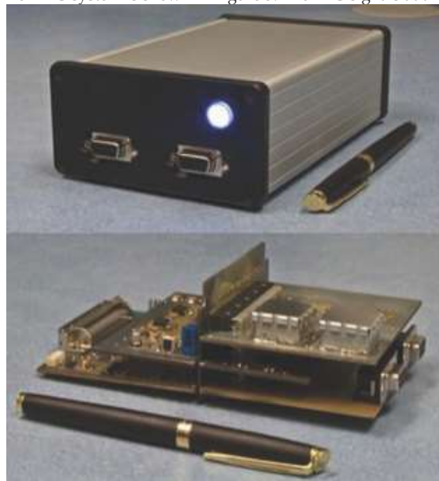
Figure 5. ZenPPG pulse oximetry processing system. The top photograph shows the front panel of the completed (all electronics are enclosed) 2-channel pulse oximetry system. The bottom photograph shows the printed circuit boards of the dual channel pulse oximetry system.
