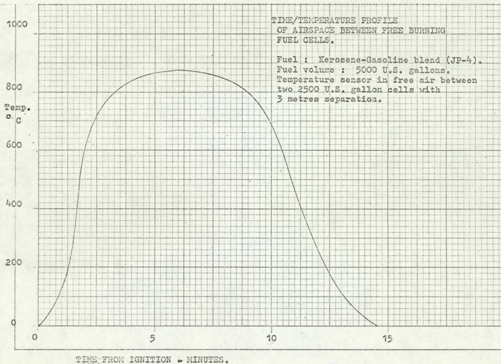
FIGURE 8. Fuel Fire Time/Temperature Profile.
