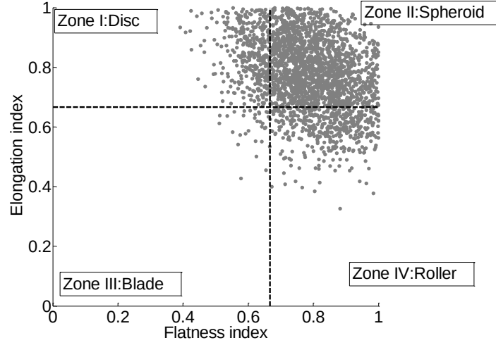
Figure 13 Elongation plotted against flatness for a representative reconstituted sample before shearing (Rec-1a), comparing with the Zingg (1935) shape classification
