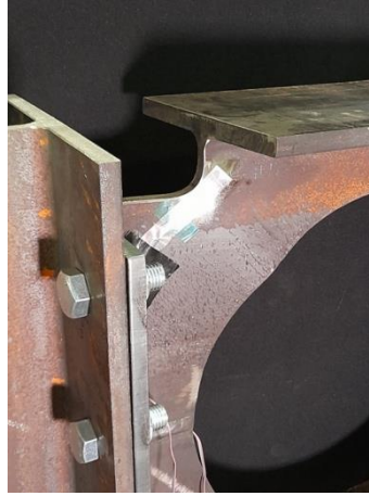
Figure A.4: Buckling at narrow end post of notched beam.
