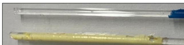
Figure 2 Photograph of the ‘dummy sensor’ (NIP) – a optical fibre coated with a material which is not imprinted and thus has no interaction with the codeine (indicated by the absence of the yellow colour), and the molecularly imprinted sensor (MIP) – giving the yellow colour.
