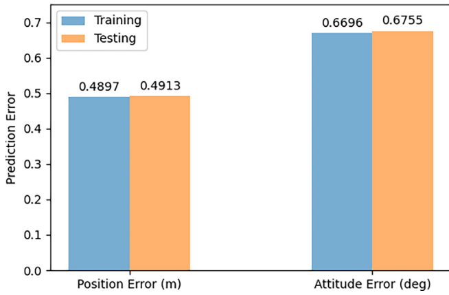
Fig. 5. The prediction accuracy of the proposed pose estimator on training and test dataset after 50 epochs. The blue bar presents the average error on training data and the orange bar represents the average error on test data. (For interpretation of the references to colour in this figure legend, the reader is referred to the web version of this article.)
