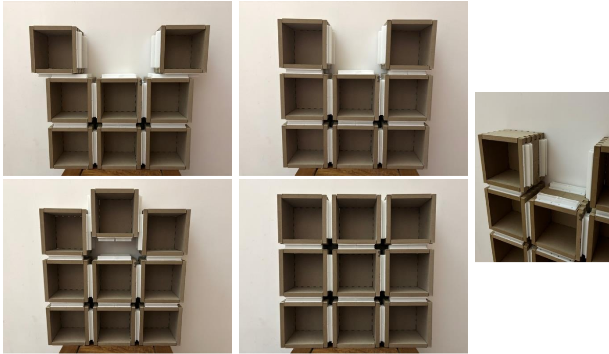
Figure 6. Illustrations of model installation and details of interlocking connections on timber modules.
