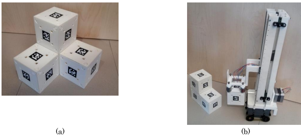
Figure 10. Prototypes of (a) the stigmergic building block and (b) the mobile robot [45]
