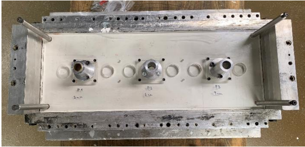
Figure 3: Pile installation guide on soil sample
