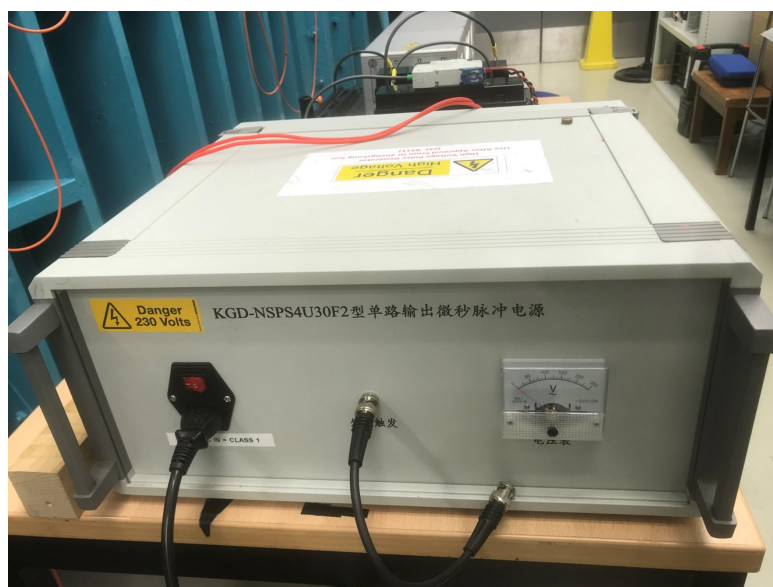
Fig. 2.2 High voltage microsecond pulse generator in the lab.
