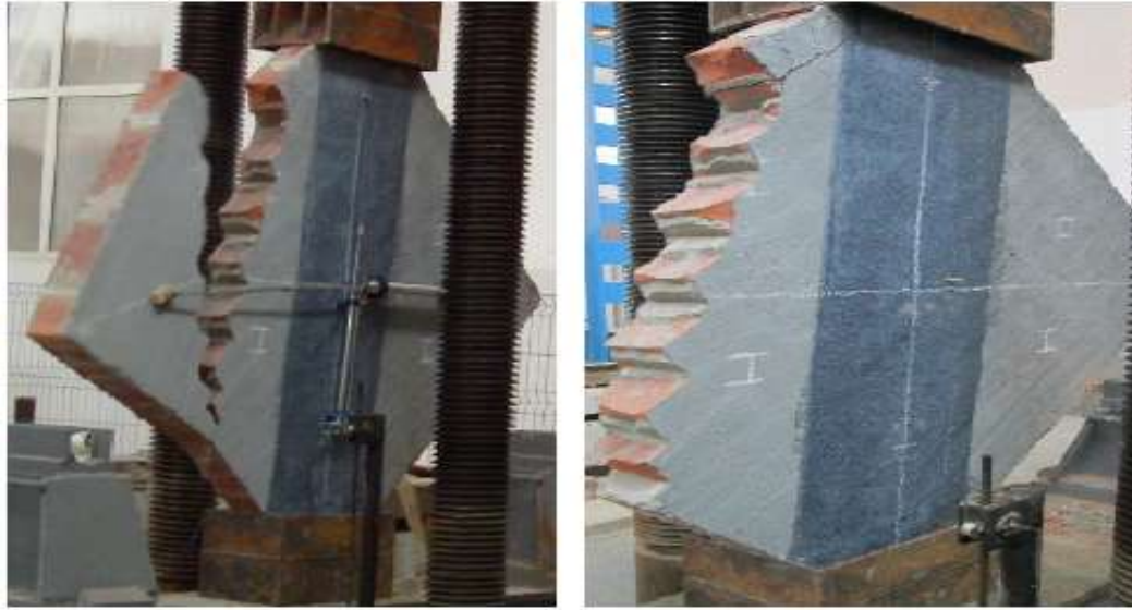
Figure 2.32: Failure mode of masonry panel with on layer CFRP (El Malyh et al. 2020).
