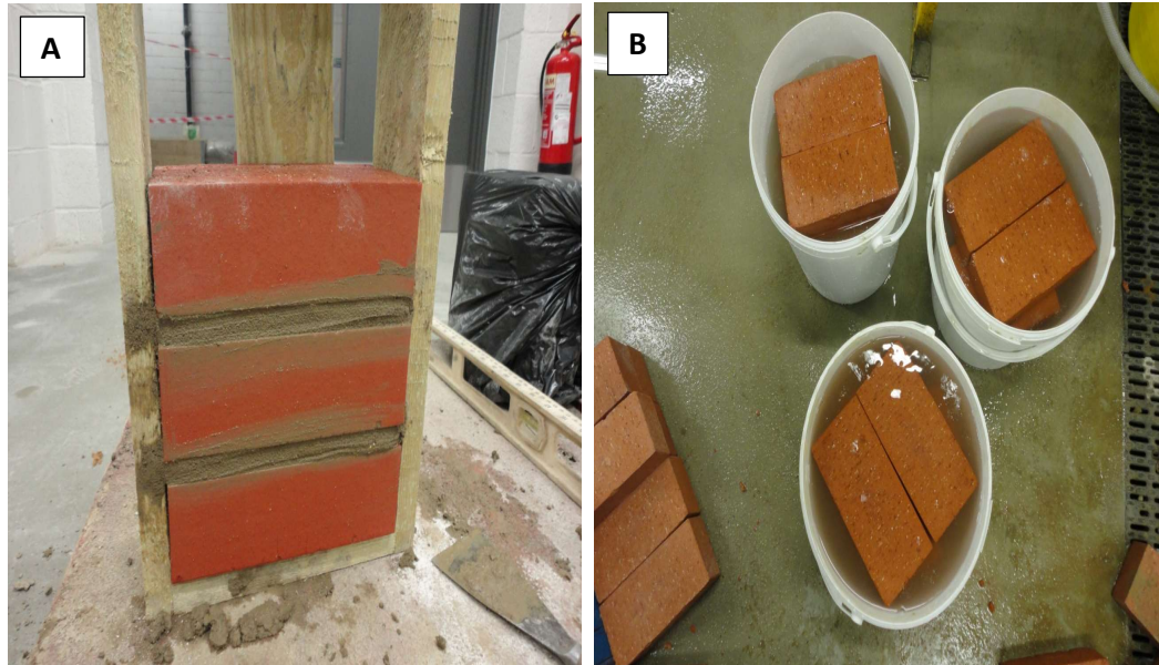
Figure 3.22: The brick units used to build the triplet samples
