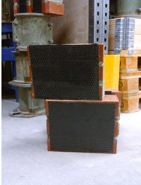
Figure 3.25: Strengthening with one layer of CFRP sheets on both sides
