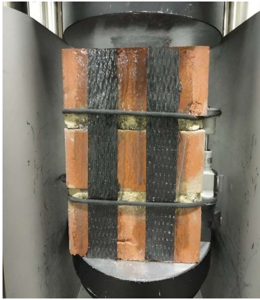
Figure 3.29: one layer of CFRP strips on both sides Figure 3.30: two layers of CFRP strips on both sides
