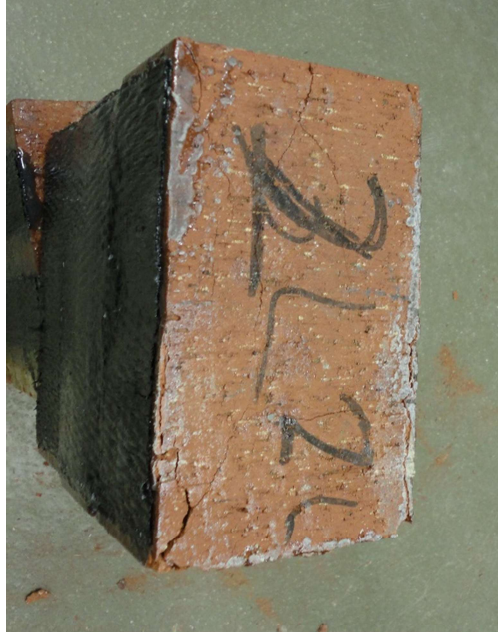
Figure 3.26: Strengthening with two layers of CFRP sheets on both sides
