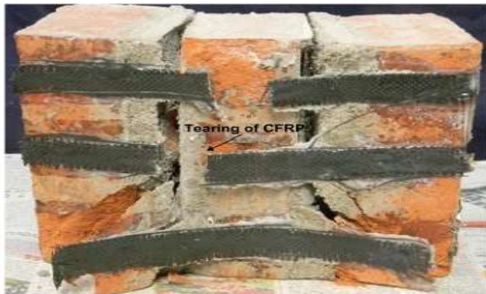
Fig. 2.30. Tearing and debonding of CFRP laminate observed in T-C200-3-2.54 triplets. Pavan and Nanjunda (2015)
