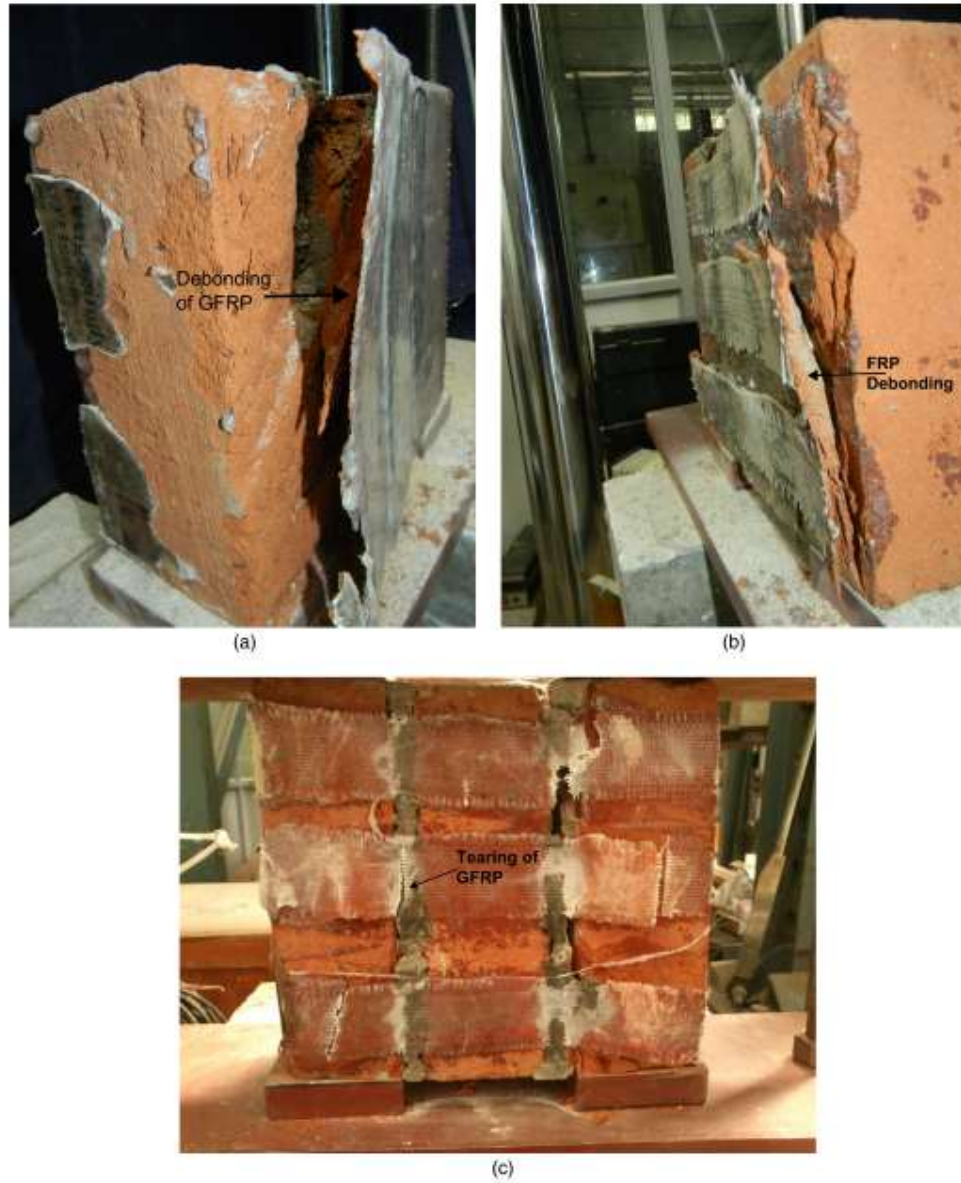
Fig. 2.28. Failure patterns of triplet specimens attached with GFRP composites: (a) debonding failure of T-G360-full triplets; (b) debonding failure of T-G600-3-4 triplets; (c) tensile rupture failure of GFRP 200 in T-G200-3-4 triplets. Pavan and Nanjunda (2015)
