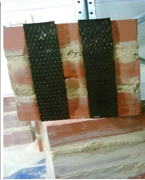
Figure 3.29: one layer of CFRP strips on both sides Figure 3.30: two layers of CFRP strips on both sides
