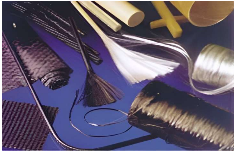
Figure 2.15. Common FRPs Used in Structural Engineering (Derias and Hacha, 2007)
