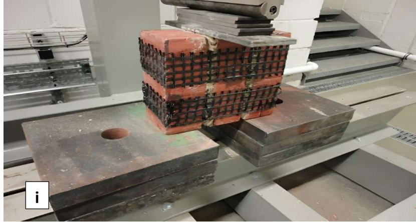
Figures 4.2: The control specimen and eight different CFRP applications on triplet masonry.
