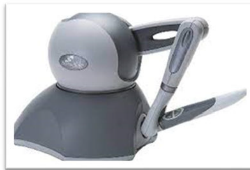
Figure 4.2 Example of a haptic stylus device
