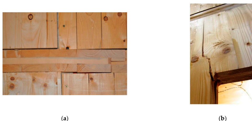
Figure 4. Timber panels damage observed in the quasi-static test of CLT buildings under large displacement: (a) embedment of wall panels into floor panels that causes the debonding of timber planks; (b) cracking in the corner of a large opening [19].
