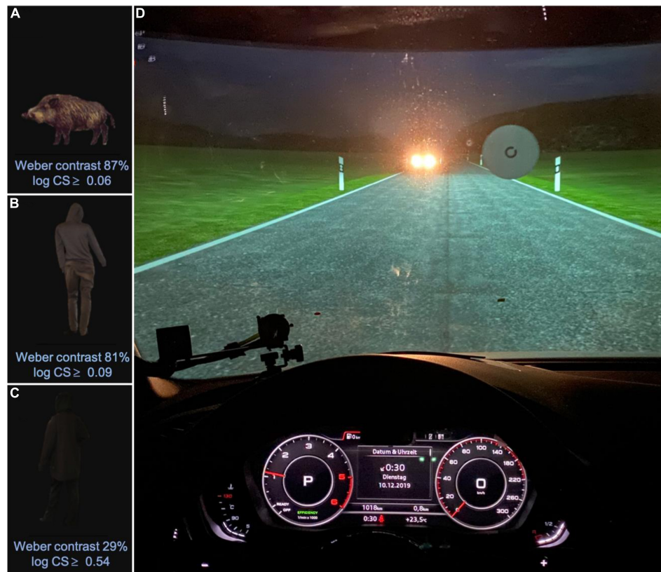
FIGURE 1 | The night driving simulator ( D ) and associated hazards ( A–C ). Hazard in Panel ( C ) may be difficult to see owing to its low contrast. Visible in Panel ( D ) is one of the Landolt Cs used to measure CS within the simulator, as well as the dipped headlights of the oncoming vehicle, which were simulated by LEDs physically moved by cable robots. The digital dashboard was fully functional and provided realistic feedback during simulated driving. Realistic auditory feedback (engine noises) was also provided. See main manuscript text for further technical details regarding the simulator. Note that when capturing the photograph shown in panel ( D ), some overexposure was required to visualize the instrument panel and compensate for the veiling glare of the oncoming virtual car. As a result, some subtle but important aspects of the lighting may not be apparent. For example, car headlights have an asymmetrical light distribution (to minimize glare to oncoming cars). So in the scene depicted here, the righthand side of the road immediately in front of the simulated car should have a more intense luminance distribution than the left. Likewise, the forward light from the simulated vehicle should decrease with eccentricity and distance from the participant. All of these details were in fact the case, but are not obvious from inspection of the photograph (e.g., apron luminance was between 1.3 and 2 cd/m 2 for the right roadside, varying as a function of distance, and between 0.6 and 1 cd/m 2 for the left).
