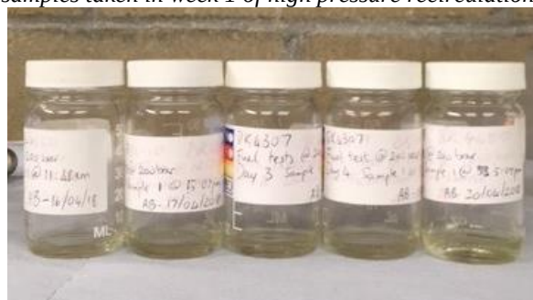
Figure 5.2.1 Fuel samples taken in week 1 of high pressure recirculation test for UV-Vis analysis
