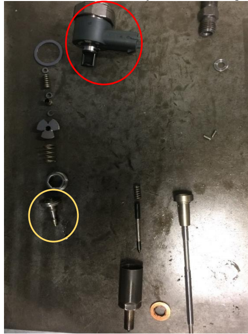
Figure 3.1.2 VAUXHALL injector solenoid spill valve
