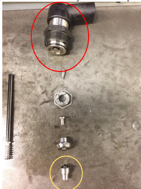
Figure 3.1.1 NISSAN injector solenoid spill valve
