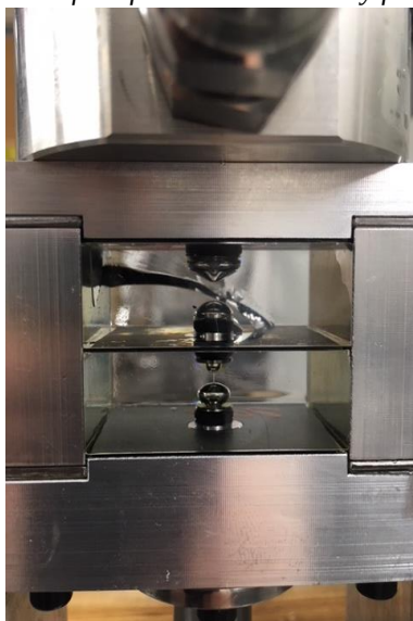
Figure 5.3.1 Downstream block of the fused silica assembly failing at 200bar upstream pressure
