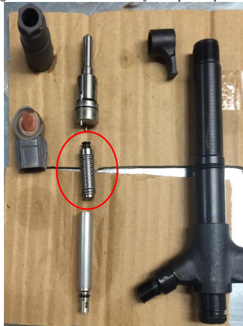
Figure 3.1.3 TOYOTA injector piezo spill valve
