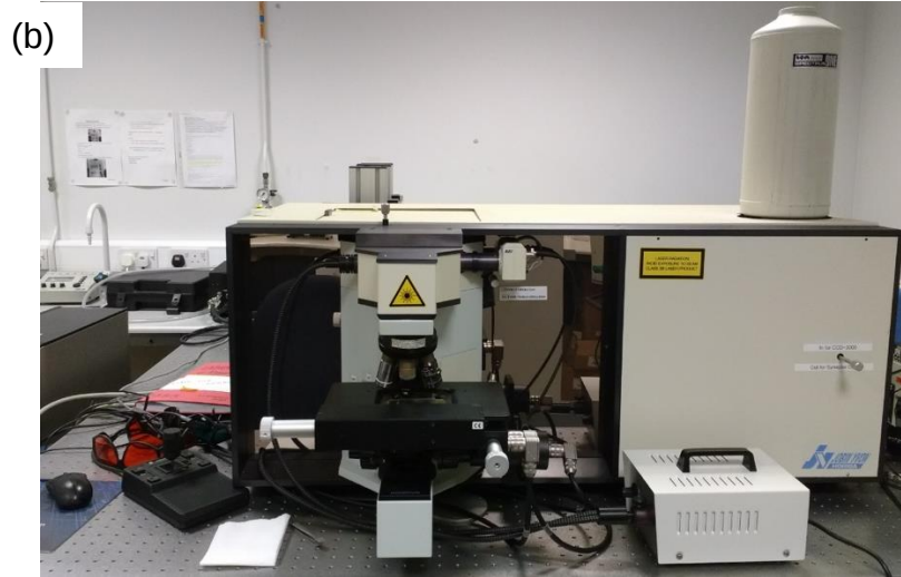
Figure 4.7: (a) Schematic representation of energy levels [202] and (b) photograph of micro Raman spectroscopy setup.
