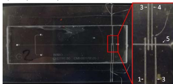
Figure 1 Microfluidic device (sensor area magnified) 1&2: CC electrodes, 3&4 PU electrodes, 5 microfluidic channel
