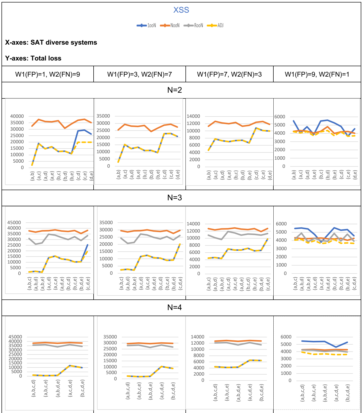
Appendix C-Figure 5 The weighted total loss (FP losses and FN losses) per diverse system configurations (1ooN, majority vote, NooN and optimal adjudication) for (XSS, N=2, 3 and 4)
