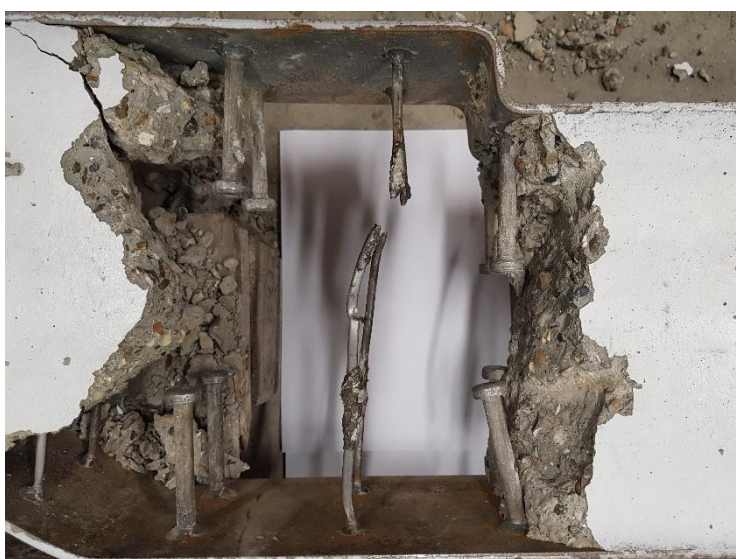
Figure 22: Steel plate local buckling of SCB1
