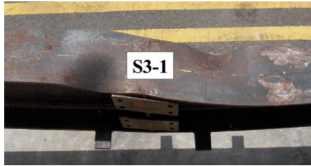
(a) Local and lateral torsional buckling observed in test (Dharma and Tan, 2007)
