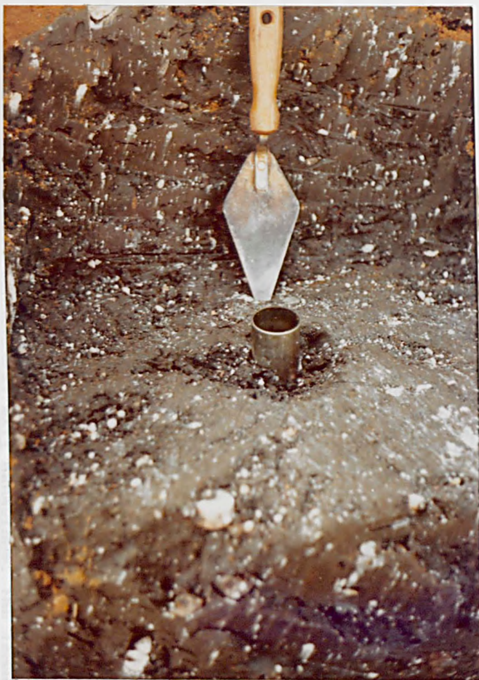
Figure 5.17 Full penetration of the 38mm sampling tube.
