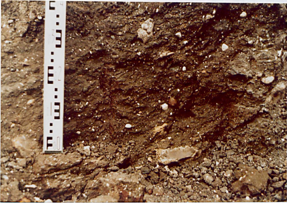
Figure 5.2 Dark grey chalky lodgement till (HH(a)) at Holwell Hyde Quarry, Welwyn Garden City.
