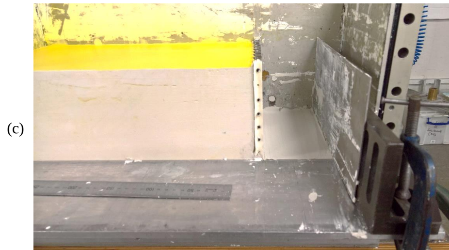
Figure 5.25 (a) Removal of treated soil from consolidation box, (b) series of angles clamped to model to accurately establish extent of ground treatment, (c) plates used to excavate virgin soil and (d) installation of lime-stabilised clay soil block
