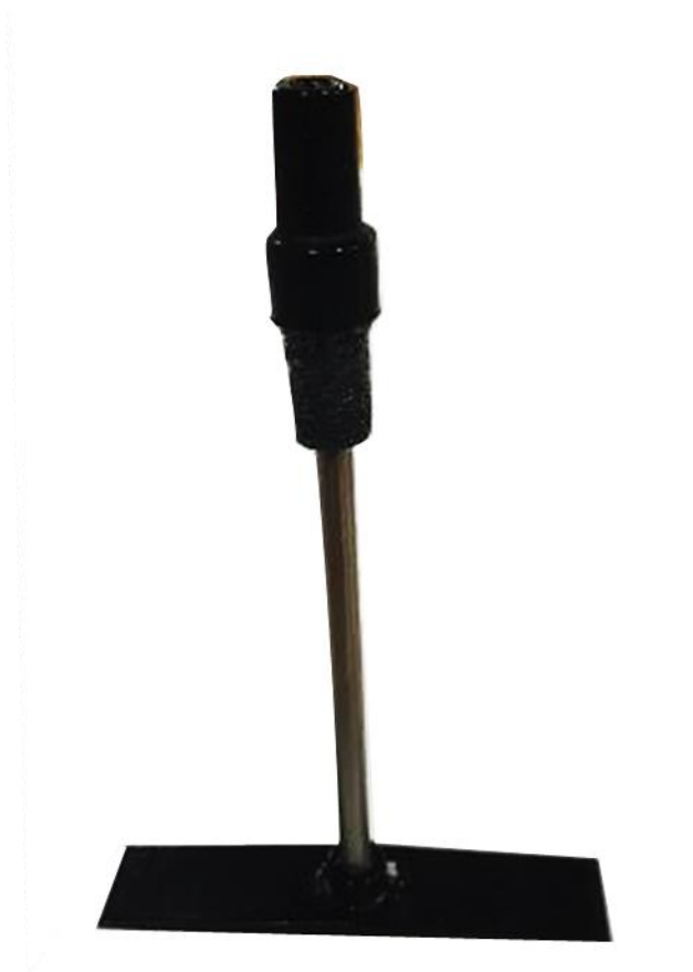
Figure 4.19 Bespoke LVDT footings for soft soil models, 50 x 10mm in plan and 2mm thick in the centre tapered to 0.5mm at the ends
