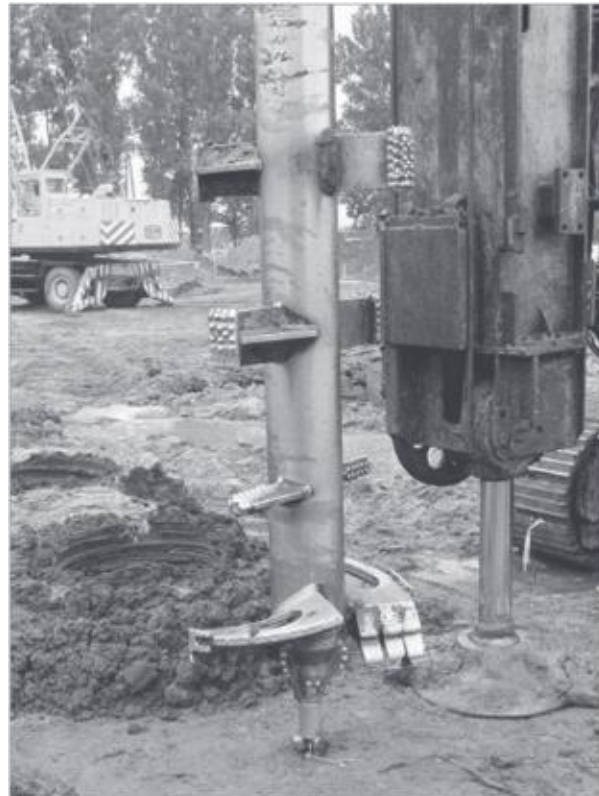
Figure 2.47 Deep soil mixing auger (Bell, 2012)
