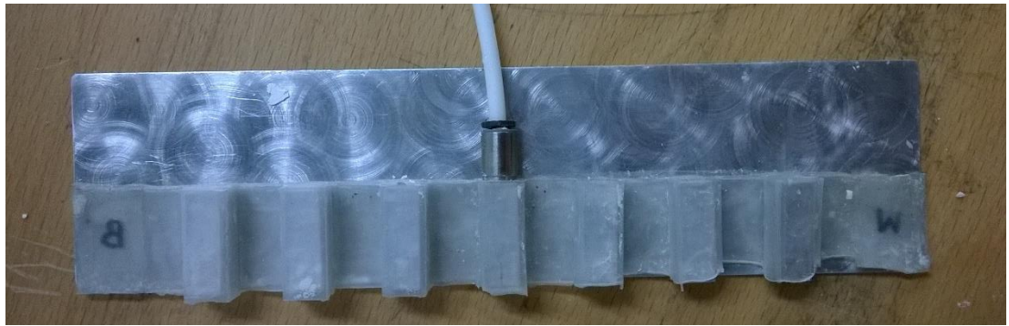
Figure 4.17 Photograph of airbag spacer with push fitting attachment for underwater test series and silicone rubber seal
