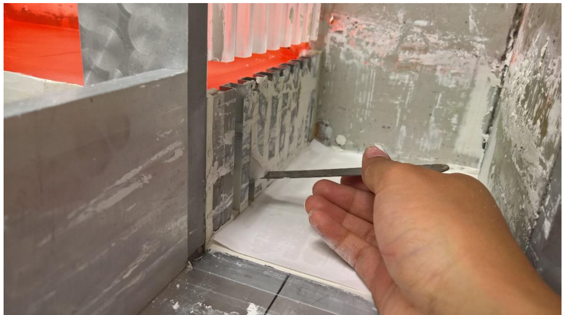
Figure 5.18 Removal of clay from between the ribs of the retaining wall
