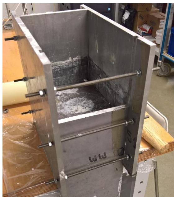
Figure 4.23 Photograph of consolidation box being disassembled by sliding out front plate
