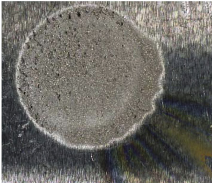
Figure 2.20: Oxide induced colour – tinting marks on grade DH36 steel (Source: Carlton, 2012)
