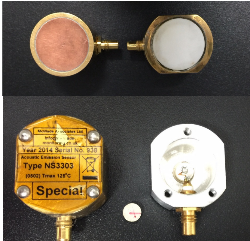
Figure 6.11: Top– PVDF and brass sensor, Bottom – Brass and aluminum Sensor along with its piezoelectric crystal sitting in its case
