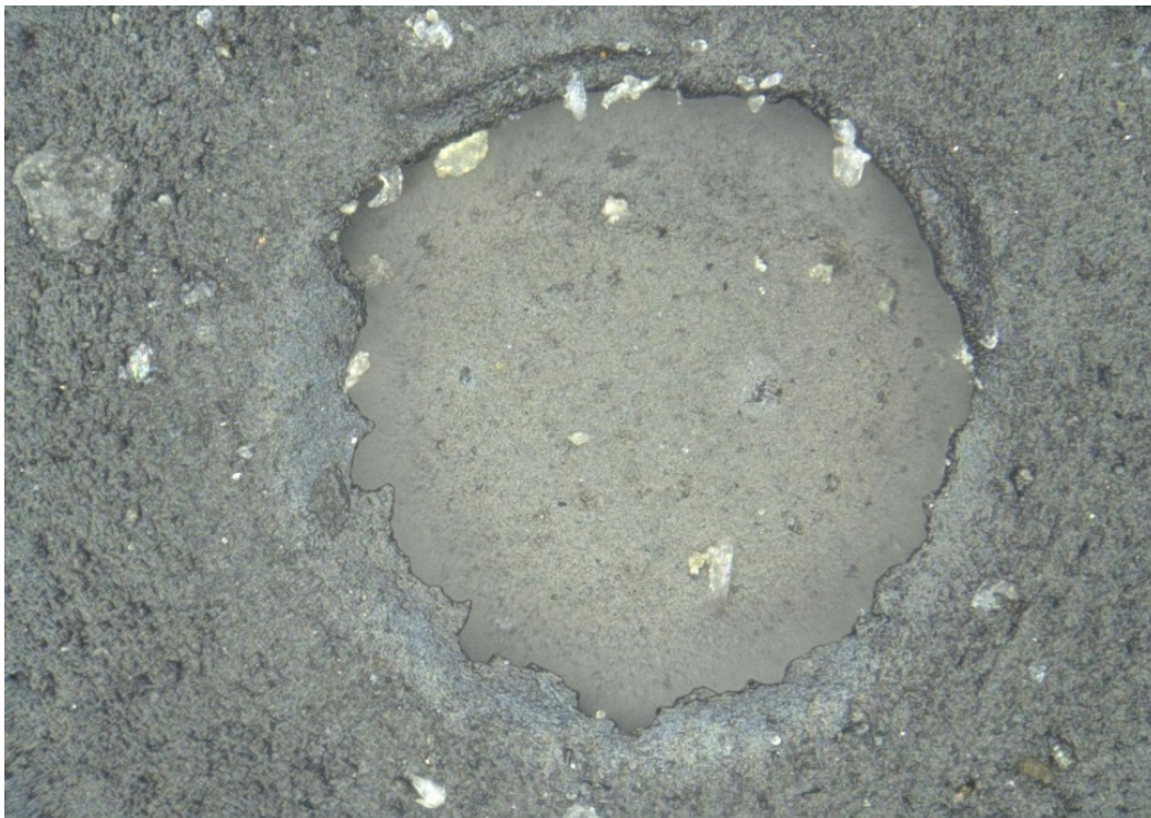
Figure 5.23: Microscopic appearance of cavitation related erosion for R coating (x500).
