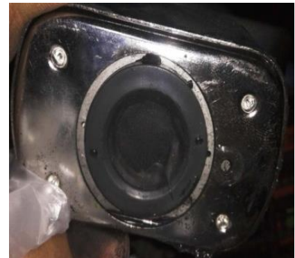
Figure 6 Laser methane sensor installed in a mine
