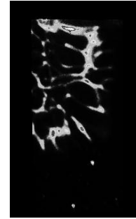
Figure 2: LII Signal from a 5 bar, \phi = 1.8 Iso-octane-Air Explosion Flame [3, 5] (Flame radius \approx 60 mm)
