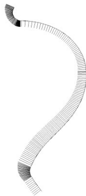
Fig 8. Clearance distribution between the rotors at the discharge rotor end
