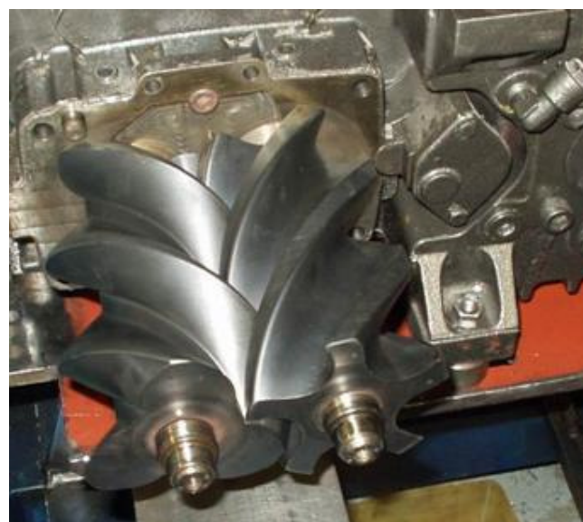
Fig. 8 Compressor rotors, housing removed
