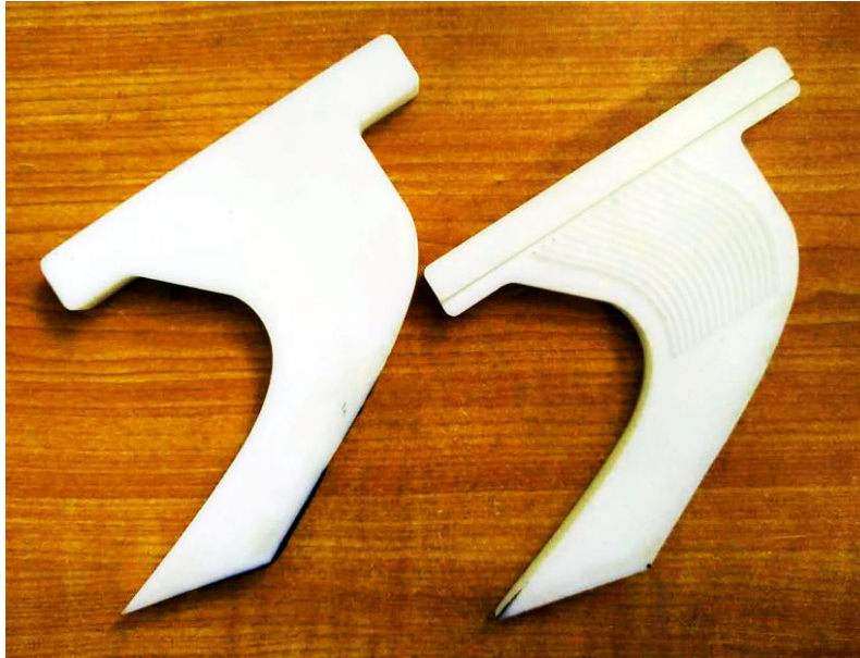
Figure 3.5: Interchangeable end-wall with smooth and ribbed surface for turbine cascade.
