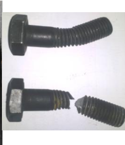
(f) Fracture of bolt
