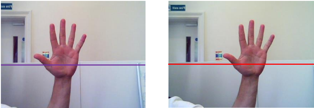
Figure 1.1 The rectified stereo image pair of a hand pose. The purple and red lines indicate respective horizontal line in the left and right stereo captures that share corresponding points.
