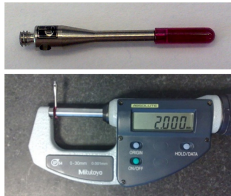
Figure 1-38 (top) 2 mm Renishaw stylus utilized as geometrical phantom for the mm size objects. (bottom) measure of stylus diameter with calibrated digital micrometre.
