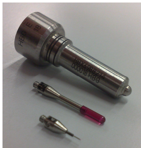
Figure 1-49 (From top to bottom) picture of the diesel injector tip that will be the object of geometrical reconstruction within this thesis, and the 2 mm and 0.3 mm Renishaw styli to visualize the scale between the three objects.
