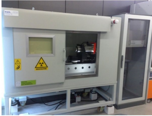
Figure 1-19 Outside view of the X-ray machine with door open; control electrical cabinet on the right side of the picture.
