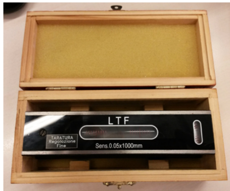
Figure 2-5 Level with a resolution of 50 micrometre per meter utilized for the drop on Teflon.
