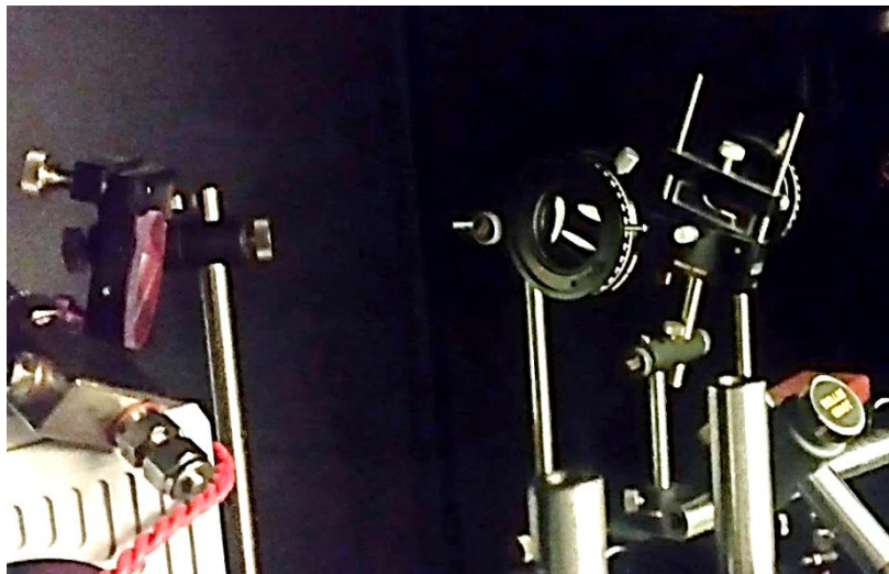
Figure 3.16: Picture showing the cylindrical telescope arrangement and the \varnothing 50mm mirror.
