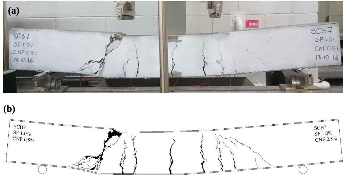
Figure 5.55. SCB7: (a) after the test; (b) crack map after the test
