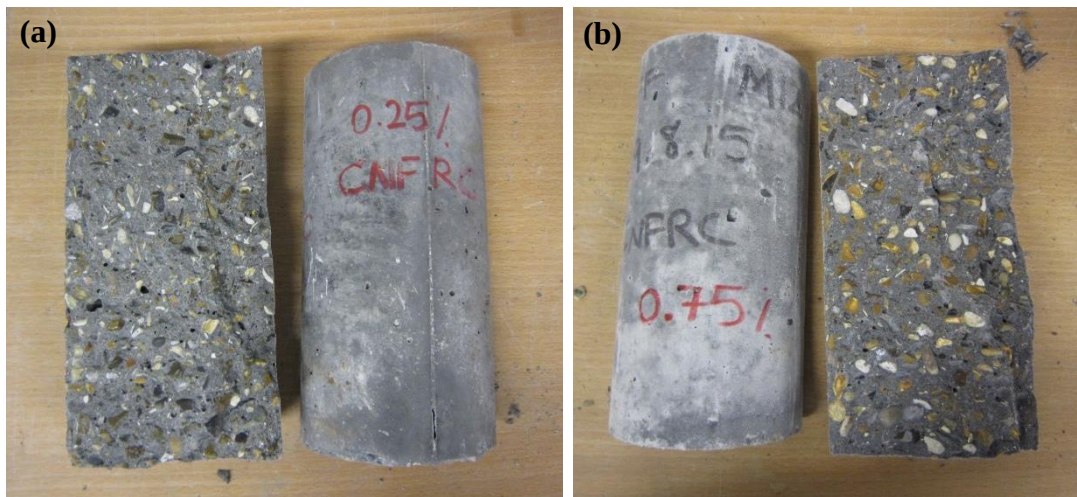
Figure 3.19. Split tensile failure of cylinders - Group B: (a) CNFRC0.25; (b) CNFRC0.75
