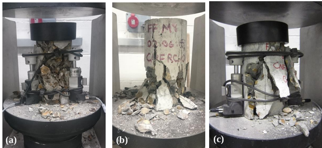
Figure 3.12. Compressive failure of: (a) PC-A; (b) CNFRC-A-0.5; (c) CNFRC-A-0.75
