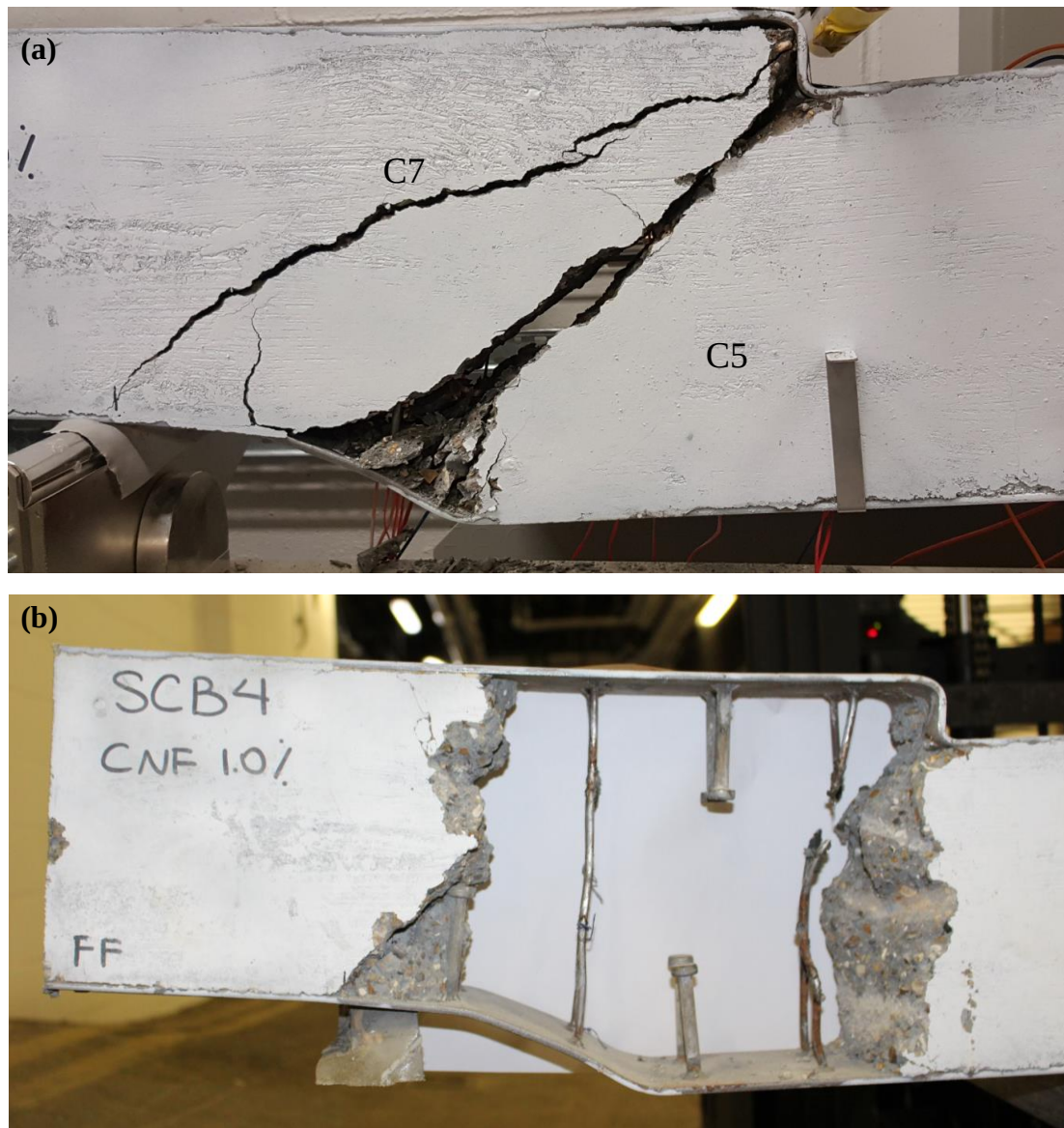
Figure 5.34. (a) Enlarged view of C5 and C7 for SCB4; (b) tie bars crossing C5 and C7 after demolition of the concrete core
