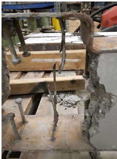
Figure 5.24. Fractured tie bars in SCB3 (east shear span)
