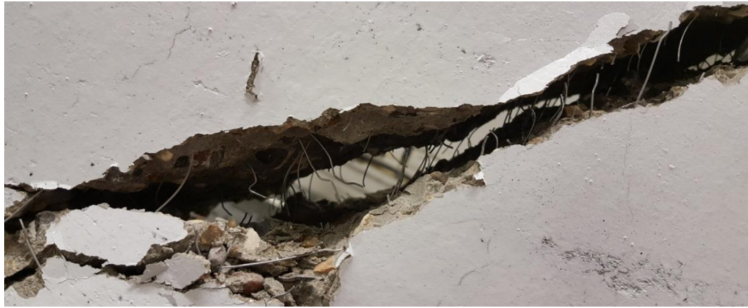
Figure 5.17. Close view of steel fibre at the crack interface
