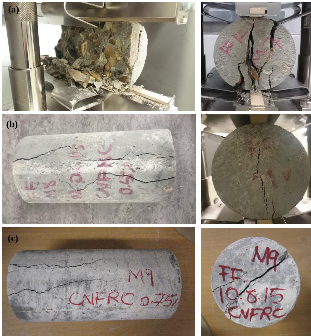
Figure 3.13. Split tensile failure of cylinders - Group A: (a) PC; (b) CNFRC-A-0.5; (c) CNFRC-A-0.75
