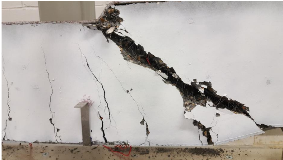
Figure 5.42. Closer view of the shear crack for SCB5
