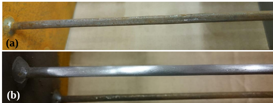
Figure 4.11. Tie bar: (a) before surface sanding; (b) after surface sanding.
